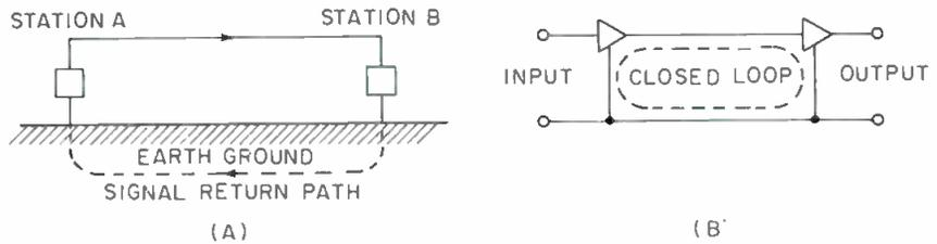
Figure 1. An unbalanced line. (A) is the physical representation and (B) the schematic one.
