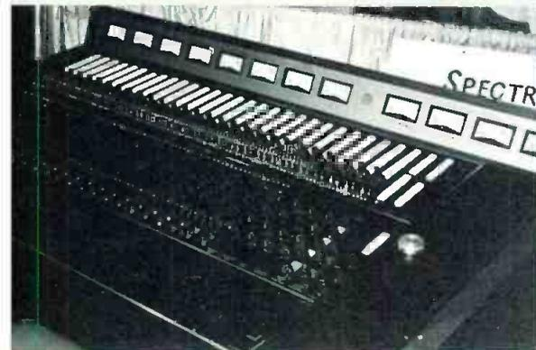
Full quad mixdown is only one of the features of Spectra-Sonics 24 in, 24 out console. Circle 62 on Reader Service Card.
