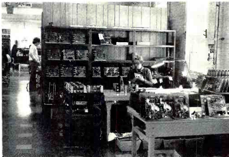
Units are being completed at this station, while behind it, completed circuit boards are stored awaiting the production of the system for which they might be destined.
