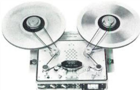
**Stellavox SP-7** The ruggedly built SP-7 is so compactly designed that you'll be amazed at how little it weighs (only 8 lbs. with tape and batteries). Wow and flutter:  $< \pm 0,07\%$ . Overall frequency response: 30 to 16,000 Hz  $\pm 2$  dB. Signal to noise ratio, weighted (ASA A filter)  $> 65$  dB stereo and  $> 70$  dB full track (at 50 mMX/mm).
