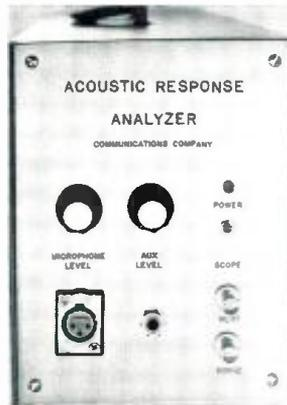
● Almost any oscilloscope may be converted into a real time audio analyzer with the ARA-412 audio response analyzer. Although it is not an impulse analyzer, it can be used to analyze all types of sound which have a less significant time framework. The device covers the audio frequency range from 40 Hz to 16 kHz, with 27 parallel bandpass filters. It has an input impedance of 100,000 ohms high level and 250 ohms microphone level.
