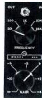
● Five selectable frequencies (50 Hz, 100 Hz, 1 kHz, 10 kHz, and 15 kHz) and a controllable level of signal output from -74 dBm to +4 dBm are offered by model 800 signal generator. The solid state generator is designed so that it may be turned on or off without introducing transients into the circuitry. All controls are located on the front panel; the unit measures a compact 3½ x 1½ x 2¾ inches.
