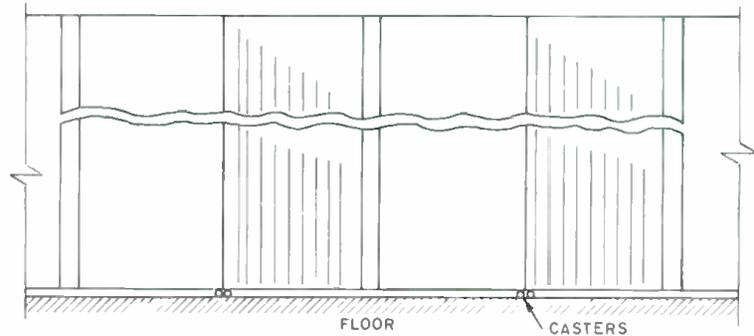
Figure 3. Details of construction of an "accordion-edge" folding partition.
