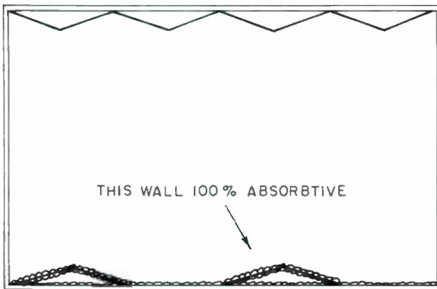
Figure 1. Illustration shows use of folding panels on sidewalls of a recording studio to provide (top) a wall which is highly reflective; (middle) to construct instrument calls; (bottom) to achieve a wall which is highly absorptive.
