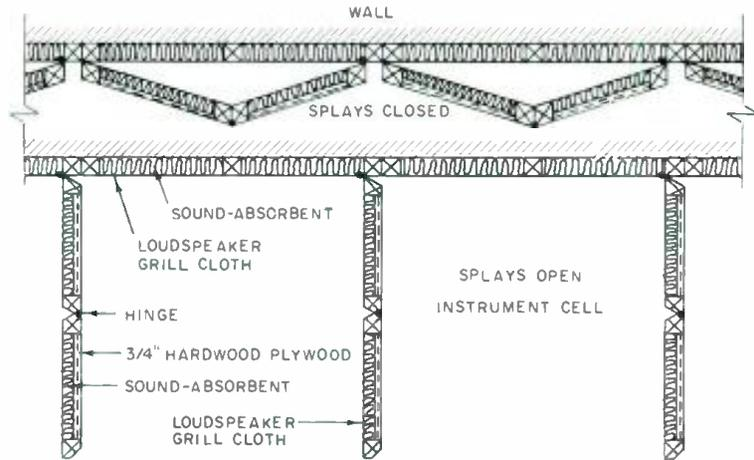
Figure 2. Details of construction of the folding wall panels shown in Fig. 1.
