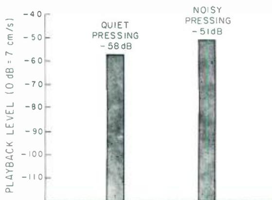
Comparison of surface noise on quiet and noisy vinyl pressings (RIAA playback, "A" weighted scale, unmodulated groove).
