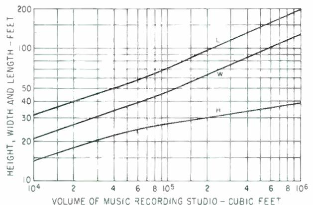
*Graph gives recommended dimensions of recording studios and shows that the height increase is slower as the length and width of a studio are increased.*
