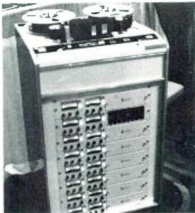
Xedit's 16 track deck fitted with Inovonics electronics.
