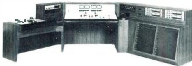
● The monitor system on this console is capable of selecting nine different points in the console system for immediate comparison of various functions without affecting the program or preview signal paths. The preview to program crosstalk is bet-
