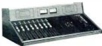
● Available in mono and stereo models, the Slide-Mod consoles have linear slide faders and completely modular construction with all active electronics on plug-in modules. The basic console frame assembly accepts up to ten input modules—either mike input or line input. All modules have momentary pushbutton activated solid state switching of audio to program audition, or cue amplifiers. Each module accepts three inputs with switching of
