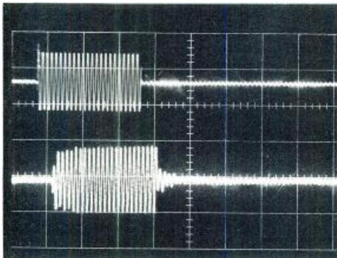
*Typical toneburst response of a medium quality domestic loudspeaker system. Upper trace: amplifier input; lower trace: loudspeaker output.*
