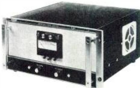
The Crown M-600 power amplifier was designed specifically for applications requiring relatively high power levels. The M-600 maintains all the exacting Crown laboratory performance standards, plus featuring built-in cooling for continuous full power operation.
