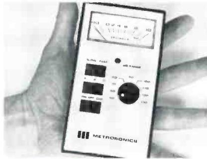
● Small enough to fit into a pocket, model db-201 is offered with an accessory clipboard providing one-hand operation. The unit's miniature microphone is mounted on a telescoping boom, which can be placed close to the sound source. db-201 covers a full 90 dB dynamic range and includes weighting networks for A, B, and C frequency response and fast or slow meter damping. The unit operates on low power solid state integrated circuits, on one battery. An accessory earphone is available.
