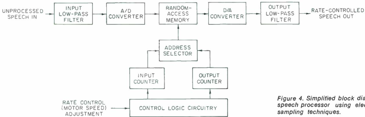
Figure 4. Simplified block diagram of speech processor using electronic sampling techniques.
