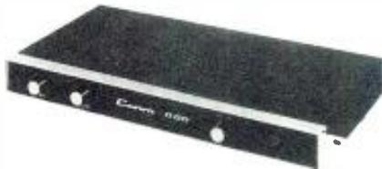
The Crown D-60 stereo amplifier, small in size, big in value and adaptability. Its uses include headphone power supply for system monitoring; ideal power for high-efficiency speakers; can be easily used in bi-amping and tri-amping situations and can be field modified to produce 25 volt monaural output power for industrial sound distribution systems.
