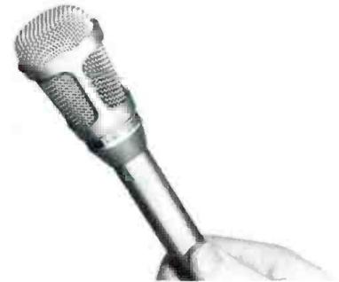
● Designed primarily for sports broadcasts and news remotes, SM82 line-level unidirectional microphone contains its own line-level amplifier, peak limiter, and 9.8V battery. Its balanced line-level output can drive telephone lines or other line-level inputs. Up to a mile of unshielded cable can be used between the mic and the broadcast equipment without equalization. Frequency response is 40-15,000 Hz. Supplied with the unit are a windscreen and a locking swivel adapter.
