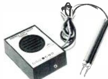
● An audible pitch, varying in tone according to the amount of resistance (0 to 50 ohms) issues from ACT-1 tester while monitoring electrical wiring and electronic circuits. The manufacturer claims complete safety for delicate components, sensitive circuits and semiconductors. Probes produce 2.5V when circuit is open, and 6mA when shorted. Powered by a 9 Vdc battery, the unit measures 2¾ x 1-3/16 x 3¾ inches. It comes complete with 30-inch probes, battery and alligator clips.
