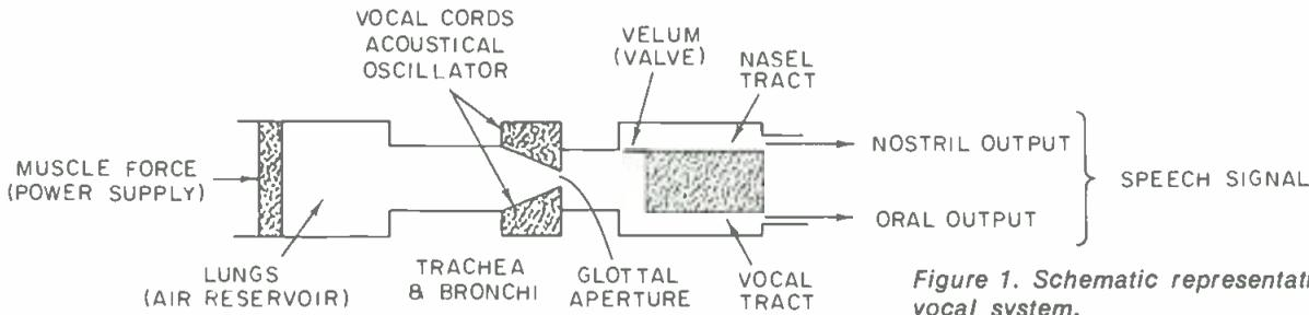
Figure 1. Schematic representation of the human vocal system.
