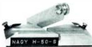
● An integrated self-sharpening shear mechanism replacing a razor characterizes this manufacturer's line of splicers. Model H-50-S, specifically for ½-in. tape, contains a precision dovetail aluminum groove which secures the tape during the splicing operation
