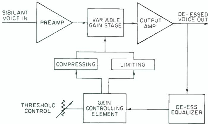
Figure 2. A simplified block diagram of a de-esser system using control-path equalization.
