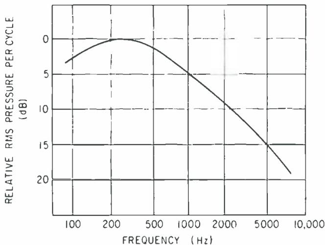
Figure 1. The spectral energy distribution curve for speech.
