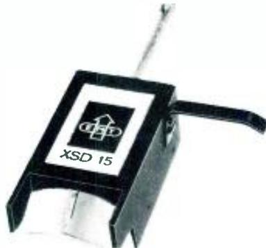
• EMT XSD-15 hand-made stereo moving-coil cartridge is built into its own shell which fits tonearms using the international plug-in configuration. A magnifying lens in the shell simplifies cueing. Each cartridge comes with its own B&K chart showing its frequency response curve from 20 Hz to 20 kHz. FIM distortion, output voltage, and channel separation.
