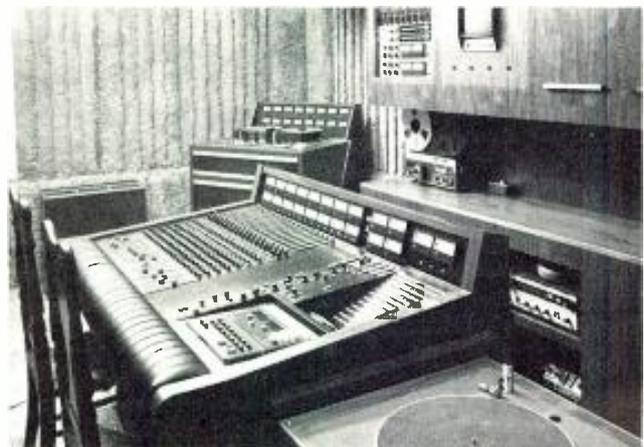
*The control room, with the 19-in, 16-out console, MCI 16-tracker, dbx, and Dolby units at hand.*
