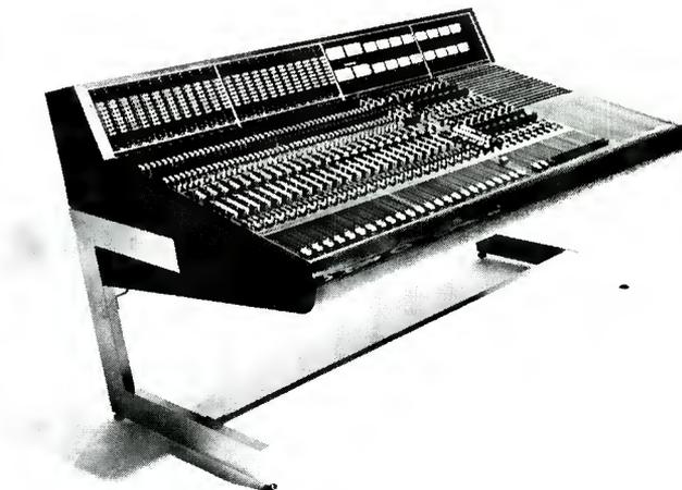
*The Trident TSM Series console featuring 24-inputs with fully removable modular patchbay.*
