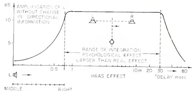
If a person sitting symmetrically between two identical noise sources L and R receive exactly the same sound impulse from both sources, it appears to him that there is only one sound source midway between L and R.
