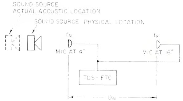
$$\text{VELOCITY OF SOUND IN FT/SEC} = \frac{D_M \text{ (HZ/LINE RESOLUTION)}}{\text{TIME/LINE} (f_F - f_N)}$$
