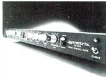
• A new audio processing device designated the SG-200 dual signal gate, was recently unveiled. The SG-200 contains two totally independent gates sharing a common power supply in one, 1 1/4-inch high, rack mount chassis. Operating controls for each gate include attack time, release time, range of attenuation, threshold, a totally silent in/out switch, and an internal/external gating command control.
