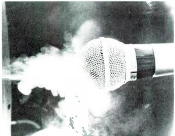
Figure 3. Synthesized pop disturbance, approaching and then striking the pop filter of a microphone.
