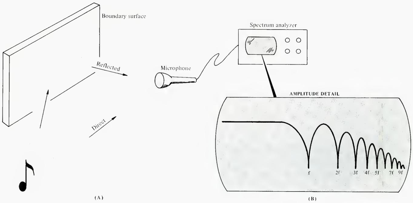
Figure 1. (A) As direct and reflected sounds are combined at the microphone, the spectrum analyzer display (B) shows the comb-filter effect. As the microphone is brought closer to the boundary, the null frequencies move beyond the audible range. (C) With the PZM diaphragm at about 25 mils from the boundary plate, any cancellation would occur far above the audio frequency bandwidth.
