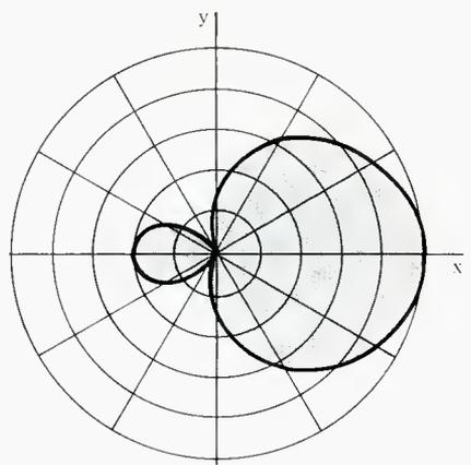
Figure 3. The polar response for a microphone with a sensitivity of  $0.3 \times 0.7 \cos \theta$ . The rear lobe (to the left of the Y axis) has a polarity reversal.
