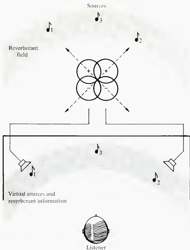
Figure 2. The Blumlein stereophonic technique. Crossed figure-8 microphones respond equally to sounds arriving from all directions.
