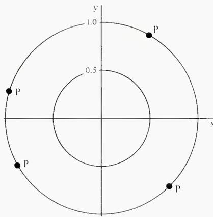
Figure 2. An omni-directional polar response. The microphone is equally sensitive to sounds at any of the points, P.
