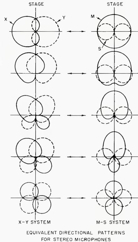
Figure 5. Various combinations of M and S microphones will produce a variety of X-Y patterns.
