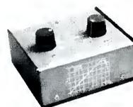
**Cat. No. 98A Noise Weighting Filter.** The Cat. No. 98A uses the CCIR/ARM characteristic and operates with an average responding meter (ordinary mil/voltmeter) to make noise measurements on tape recorders, tapes, FM receivers, etc., which correlate closely to the subjective effect of the noise. The CCIR/ARM characteristic is in wide use throughout the world; the Cat. No. 98A can be used for testing both professional and consumer audio equipment.
