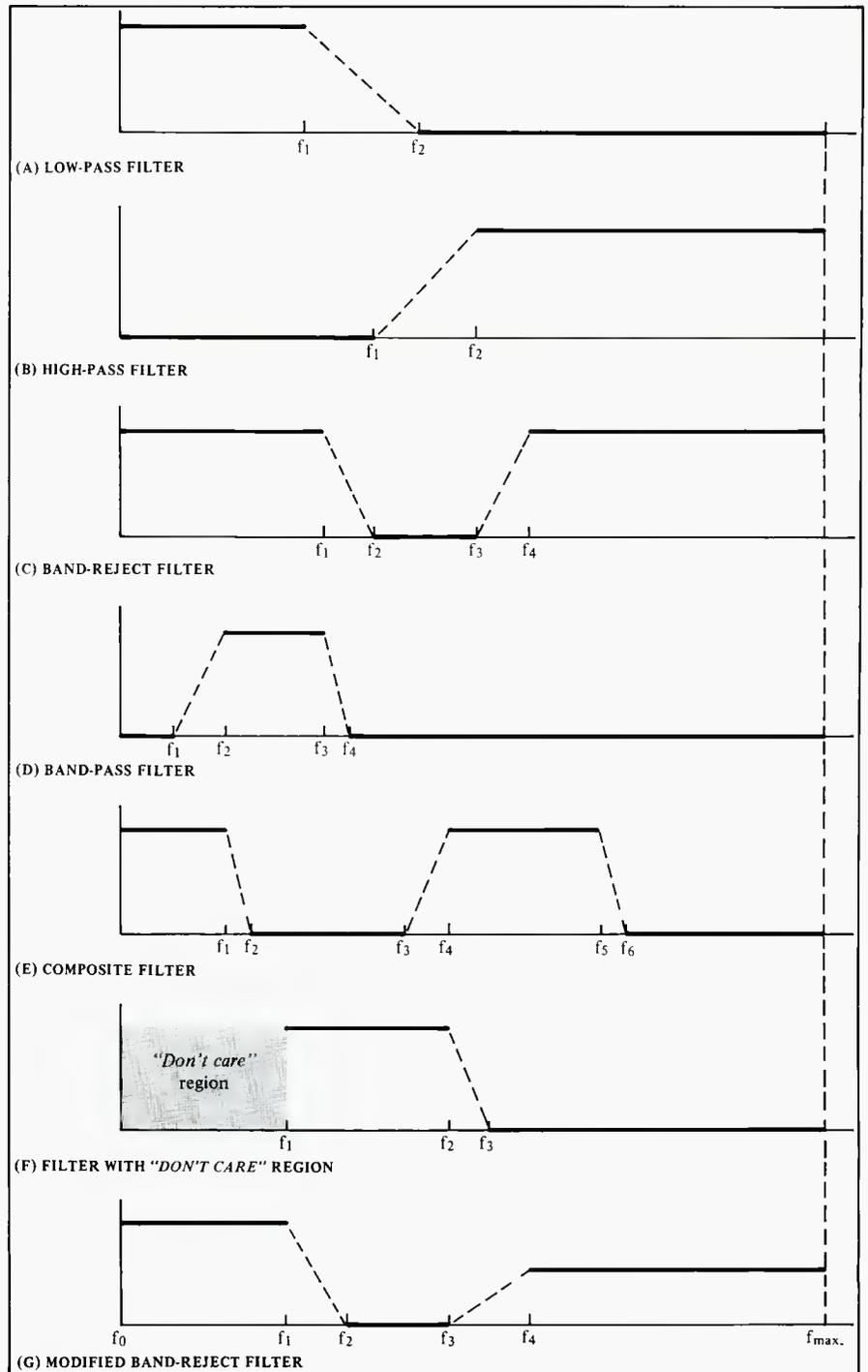
Figure 1. Target values for various types of filters.
