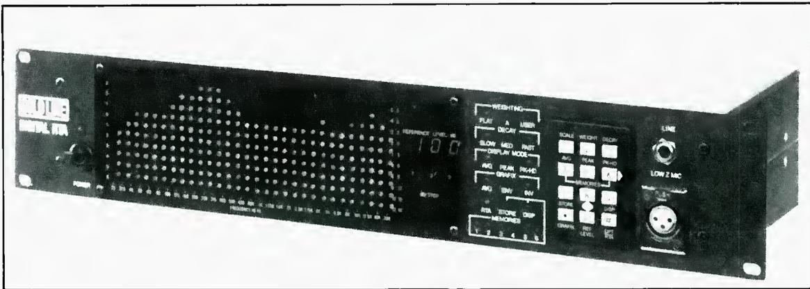
**I**F YOU DO A LOT of rock gigs and you're looking for a real-time analyzer for your P.A. system, the Gold Line 30 may be just what you're looking for. The Gold Line 30 is a digitally controlled, one-third octave analyzer with a substantial list of additional features. It's designed for quick, easy operation, making it a real time saver on the road.
