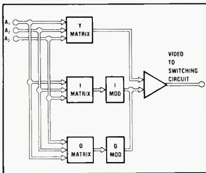
Figure 1: Samples of the stereo difference signal (L-R), shown here as A1, A2 and A3, are processed much as R, G, B color signals would be sampled by the Grumman Color Encoder.
