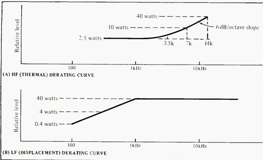
Figure 2. High-frequency de-rating curves.
