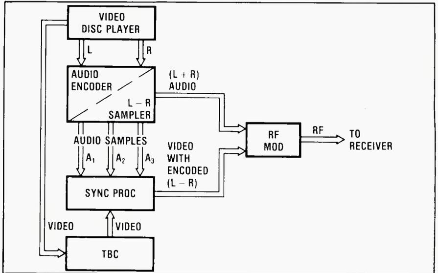
Figure 6. Block diagram of the Grumman stereo audio encoding process.
