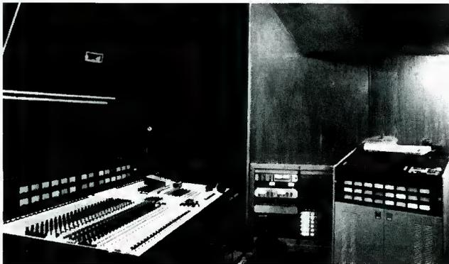
*The LEDE control room at Telearte with time-aligned monitors, Sphere console, and Ampex ATR-124 multi-track recorder.*
