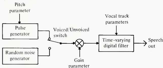
Figure 2. Block diagram of a simplified model for speech synthesis.
