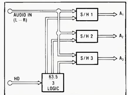
Figure 3. Sample & Hold (S/H) circuits sample the amplitude of the stereo difference (L-R) signal three times during each horizontal line of video.
