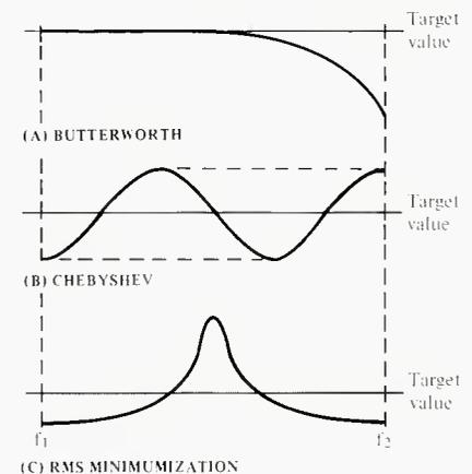
Figure 2. In each of these filter types, the actual response varies from the straight-line target value.
