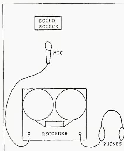
*Figure 2. The setup for leakage experiments.*
