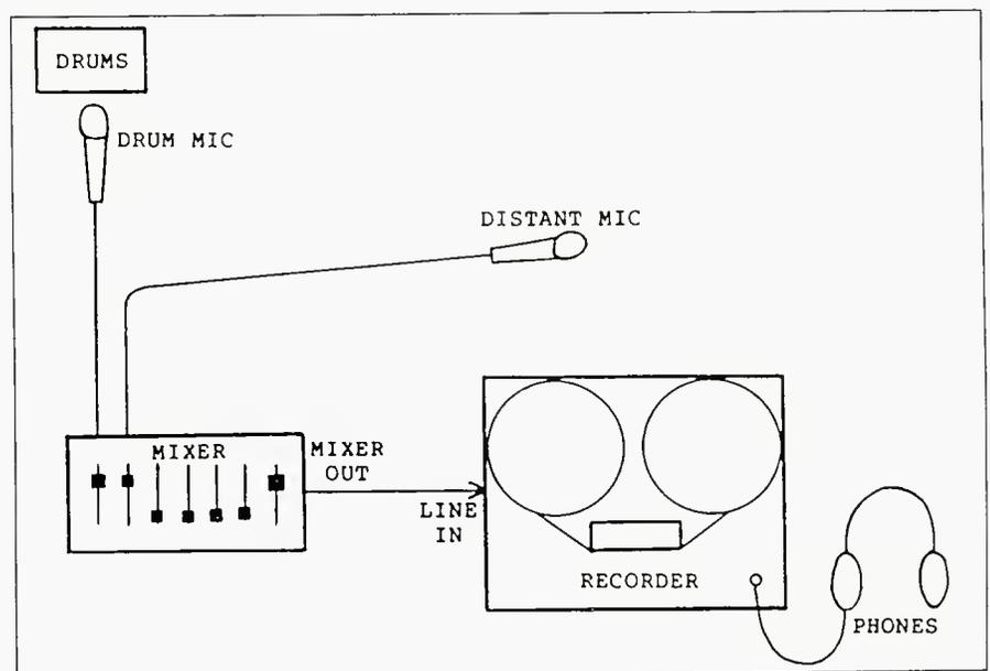
recording level. Play back the tape. Even though you recorded at a moderate level, you're likely to hear distortion caused by the microphone signal overloading the mic preamp in the tape recorder. Insert a pad in the microphone cable (such as a resistive voltage divider with 20 dB loss) and repeat the recording. The distortion should be eliminated.
