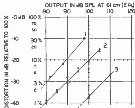
Distortion versus output for three speakers. (1) is a direct-radiator speaker in a 1-cubic-foot enclosure. (2) is a direct-radiator speaker in a 1½-cubic foot enclosure. (3) is a large-horn woofer design speaker occupying 16 cubic feet of space.
