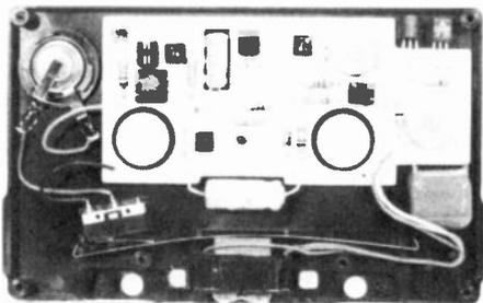
• Inside the head demagnetizer is a printed circuit board with a rather complex and sophisticated electronic circuit. Battery is in the upper left-hand corner of this photograph.
