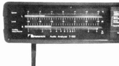
• Bar graphs are created when individual plasma cells glow. From a distance the cells appear to merge into a solid light bar. Here the bottom graph indicates  $-10.5$  dB, while the top indicates  $-14$  dB.
