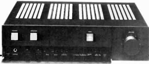
Yamaha's A-1 integrated amp has a DISC switch which is able to electrically direct-couple the phono pickup to the output power amplifier. Direct-current equalizer improves transient response. \$595. Circle Number 101.
