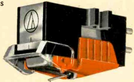
Audio-Technica cartridges have been widely-acclaimed for their great sound, and for good reason. Our unique, patented\* Dual Magnet construction provides a *separate* magnetic system for *each* stereo channel. A concept that insures excellent stereo separation, while lowering magnet mass. And the AT12XE features a tiny 0.3 x 0.7-mil nude-mounted elliptical diamond stylus on a thin-wall cantilever to further reduce moving mass where it counts. Each cartridge is individually
