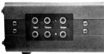
• All connections are made to phono jacks on a side panel. The scope connections permit visual observation of the T-100's test and signal output(s).
