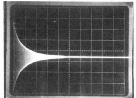
• When in use, the HD-01 applies this rapidly decaying alternating field to the recorder's R/P head. It is the decay of the field which is responsible for demagnetization taking place.
