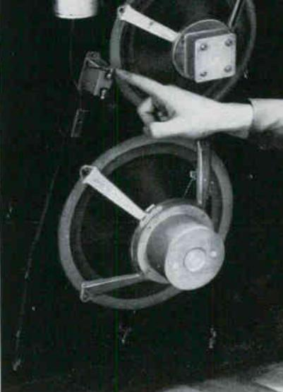
A simple capacitor acts as a crossover device by blocking the bass from reaching the upward-pointed tweeter.
