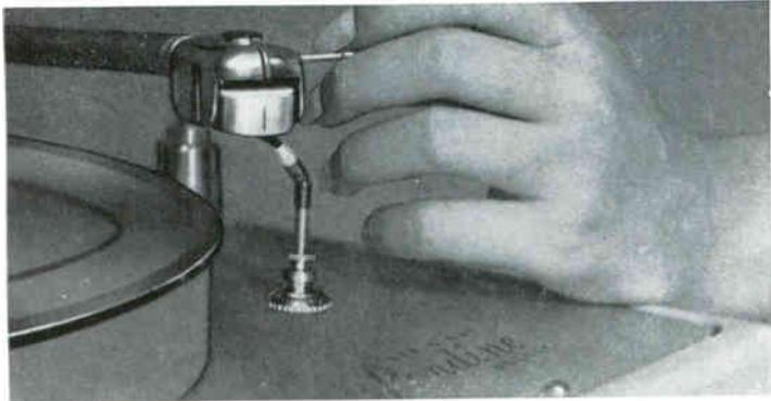
"Dirt, plain or otherwise, comes as natural to your stylus as to a pig: they just dig it up." A swipe from the KleeNeedle Stylus Brush keeps it from bunching.
