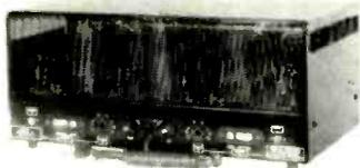
power amplifier without output transformers. The Model H-3 is rated at 50 watts per channel with a 15- or 16-ohm load and has a frequency response of +0, -0.5 db from 5 to 90,000 cps. The signal-to-noise level is better than 90 db below 50 watts. Intermodulation distortion is less than 0.05 per cent at 50 watts; harmonic distortion is less than 0.2 per cent at 50 watts (rms) output. The H-3 is unconditionally stable with any type of load, which makes it ideal for driving
