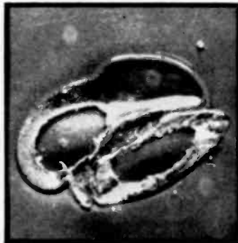
Dropouts can be caused by an oxide clump in the tape coating, shown in frontal (left) and cross-sectional (center) photomicrographs. A blister in the tape backing (right) is reflected in the coating and can cause not only dropouts, but also oxide flaking.
