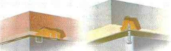
*Common staples can work themselves loose, which is why Pioneer uses aluminum screws to mount the base plate to the base.*
