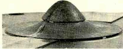
A pulsating sphere represents one ideal of loudspeaker design. Such a speaker could be made any size desired and would still have completely omnidirectional output at all frequencies. For use close to a room wall, a pulsating hemisphere would be equivalent.
