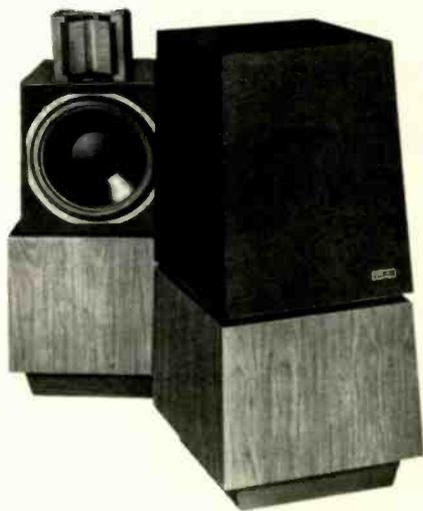
air motion transformer; frequency response 35-23,000 Hz  $\pm 3$  dB; crossover at 1000 Hz; max. input 375 W clean music power; 6-ohm nominal imp.; 120° horizontal dispersion; 30° vertical dispersion; sensitivity 87-dB SPL/W/m; mid-range presence control; oiled walnut finish with black-brown grille; 35.25" H x 16.25" W x 16.25" D ..... \$450.00
