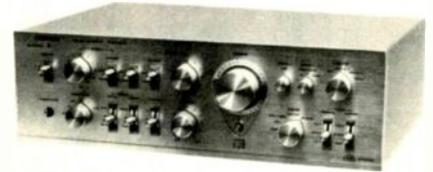
47,000 ohms (phono 2), 150 mV/47,000 ohms (aux., tuner, tape), 150 mV/82,000 ohms (tape DIN); phono overload 370 mV (1 kHz); output level/imp. 150 mV/47,000 ohms (tape), 30 mV/82,000 ohms (tape DIN); frequency response 20-20,000 Hz  $\pm 0.18$  dB (phono), 10-70,000 Hz  $\pm 1.5$  dB (tuner, aux., tape); automatic protection circuit; high and low filters; tone controls with turnover frequency selection; 41-position detent volume control; 5.7" H x 17.4" W x 14.4" D ..... \$449.95
