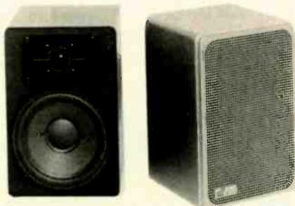
excursion woofer and 1" soft-dome tweeter; frequency response 68-20,000 Hz  $\pm 3$  dB; crossover at 2500 Hz (12 dB/octave); efficiency 90-dB SPL/W/m; rated input 50 W rms; min. input 10 W rms; 4-ohm imp.; brushed satin finish; aluminum enclosure (black or silver anodized) with aluminum grille; 8.67" H x 5.9" W x 5.7" D ..... \$140.00
