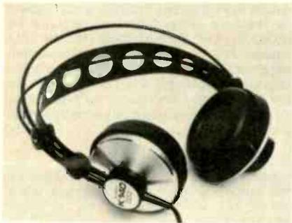
600 ohms  $\pm 20\%$  imp. over 20-20,000 Hz; sensitivity 15  $\mu\text{bar/V}$  (97.5 dB SPL); power requirements 0.75 mW (0.67 V) for 10  $\mu\text{bar}$  (94 dB SPL), 50 mW (5.5 V) for 80  $\mu\text{bar}$  (112 dB SPL); max. continuous power for 1% THD or less at 100 Hz 240 mW (12 V) for 119 dB SPL per system; supplied with 3-m four-conductor cable and  $\frac{1}{4}$ -in phone plug; 175 g. . . . \$34.50
