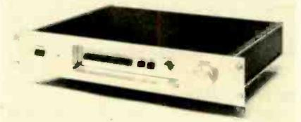
class-A symmetrical push-pull circuit; ring-emitter transistor in head-amplifier section;
