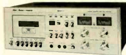
servomotor and one d.c. governor motor; three ferrite heads; wow and flutter 0.04% wrms; S/N 64 dB (Dolby on); channel separation 40 dB; signal crosstalk -70 dB; frequency response 30-15,000 Hz  $\pm 3$  dB (normal tape), 30-18,000 Hz  $\pm 3$  dB (CrO<sub>2</sub> tape); THD at 0 VU 1.4%; tape speed variation  $\pm 0.8\%$ ; fast-winding time 84 sec; two VU meters and peak-indicating LED; input/imp. 0.2 mV/600 ohms (mike), 100 mV/100,000 ohms (aux., FM Dolby); output/imp.
