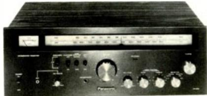
0.8%; features magnetic and ceramic phono inputs; speaker switching; mic mixing; 41-step volume control; detented bass and treble controls; FM usable sensitivity (IHF) 2  $\mu$ V; distortion 0.3% mono, 0.4% stereo; selectivity 55 dB; stereo separation 40 dB at 1 kHz; S/N 68 dB; AM usable sensitivity 100  $\mu$ V/m; selectivity 25 dB; image rejection 40 dB; i-f rejection 40 dB; 7" H  $\times$  19" W  $\times$  12 $\frac{1}{4}$ " D ..... \$199.95
