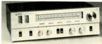
lights; FM muting; FM section: sensitivity 3  $\mu$ V; capture ratio 1 dB; AM response -50 dB; i-f response -110 dB; image response -110 dB; stereo separation 47 dB (1 kHz); hum and noise -75 dB; AM section: sensitivity 200  $\mu$ V/m (rod antenna); image response -65 dB; i-f response -50 dB; hum and noise -60 dB; 5 $\frac{1}{2}$ " H x 18" W x 13 $\frac{1}{2}$ " D ..... \$599.95
