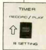
**Timer Setting** for absent recording. Now you can record Janis Joplin at home while you're out listening to Mozart. Just use the PC-3060's timer setting switch with your own timer. Recording will begin automatically at the time you set. The Auto Stop mechanism will turn it off at the end.
