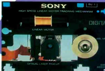
SONY'S CD PLAYER REFINEMENTS INCLUDED UNILINEAR™ CLOCK CIRCUITRY, PLUS THE FIRST 8X OVERSAMPLING FILTER AND 18-BIT CONVERTERS. WE ALSO CREATED DIGITAL SYNC™ CIRCUITRY, ONE-BIT PULSE CONVERTERS, AND THE LINEAR MOTOR LASER TRANSPORT SHOWN. THE TRANSPORT WAS THE FIRST TO CUT TRACK ACCESS TIME TO UNDER ONE SECOND.
