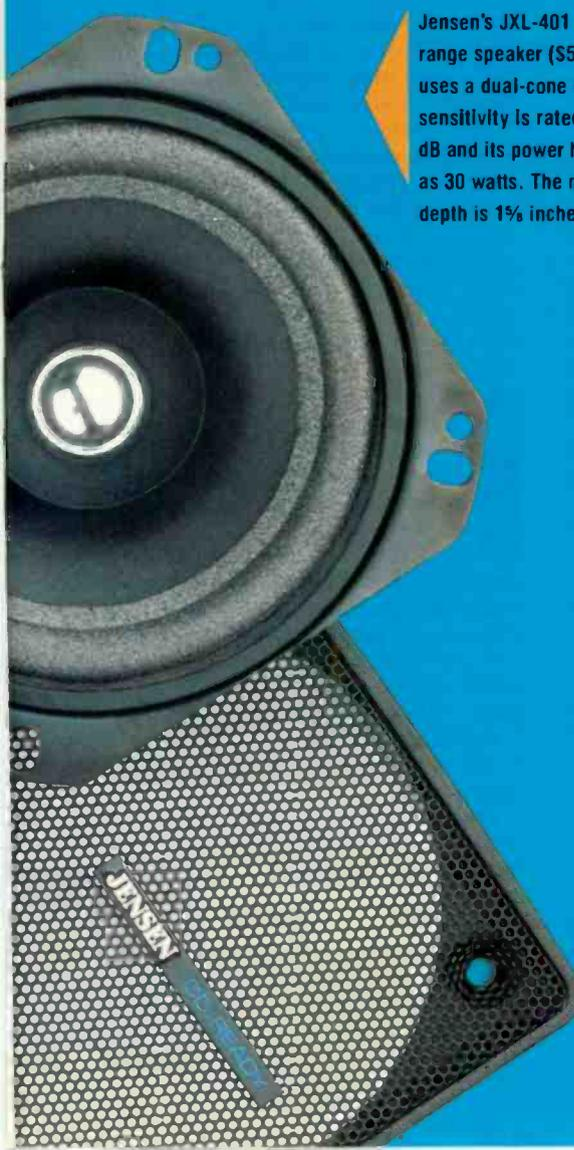
Jensen's JXL-401 full-range speaker (\$50 a pair) uses a dual-cone driver. Its sensitivity is rated as 88 dB and its power handling as 30 watts. The mounting depth is 1 1/4 inches.
