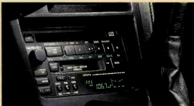
Bose sound system as standard equipment. Tight interior quarters limited the designers to only four loudspeakers: ported bass-reflex enclosures in the front doors with 4½-inch full-range drivers, a rear-mounted 2½-inch Twiddler for the center channel (or cellular phone), and a ported-enclosure 4½-inch full-range driver in the firewall. The head unit is an Alpine cassette tuner. Maximum power is 165 watts, and a trunk-mounted six-disc CD changer can be added as an option.
