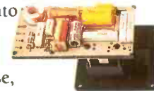
Advanced crossover network manufactured with precision capacitors and resistors.
