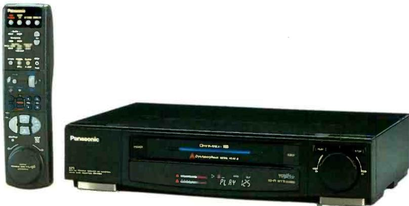
**Panasonic's VHS Hi-Fi PV-4464 (\$549) features cable-box-compatible VCR Plus recording, over-size on-screen menus, automatic digital tracking and picture adjustment (for worn tapes), and a jog/shuttle dial on both its front panel and its universal remote control.**
