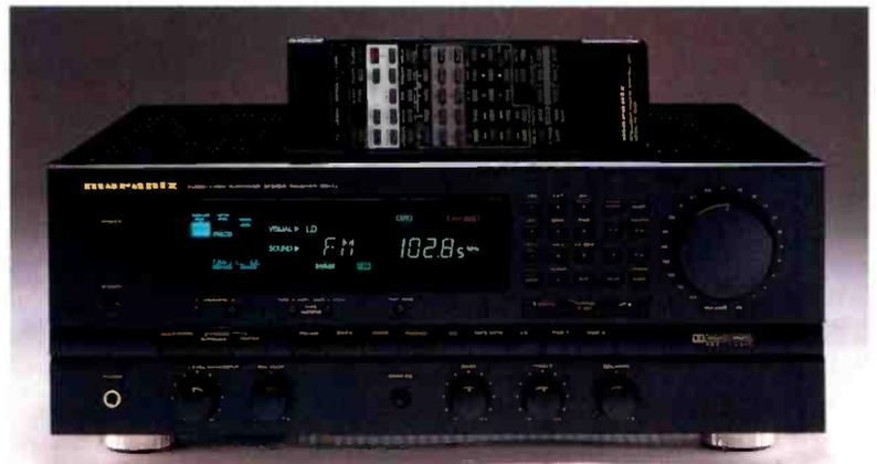
Besides Dolby Pro Logic surround sound and the other usual accoutrements of a contemporary A/V receiver, the Marantz SR-82 (\$899) has a multiroom mode that uses the surround-channel amplifiers to drive loudspeakers in a remote room, enabling independent source selection and volume control.
