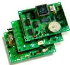
Advanced surface-mount semiconductor technology packs the processing power of a personal computer into a space the size of a light switch. A lithium back-up battery protects the program memory for up to ten years.
