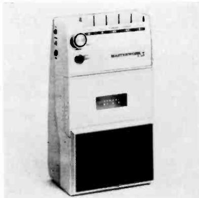
matic level control; will operate on batteries or 117 V a.c. line. Playing time up to 90 min. 4 7/8" w. x 9" x 3 1/2". Has dynamic mic. ....\$69.95
