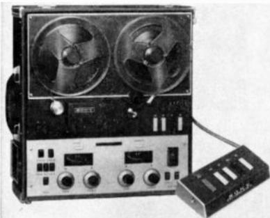
ips) design; features special "Electro-Bilateral" head construction; three motors; complete remote control; sound-on-sound; mic & line mixing; tape and source monitoring; 3" vu meters; response 50-15,000 Hz ±2 dB @ 7½ ips; signal-to-noise ratio 50 dB; flutter & wow less than .15% @ 7½ ips; has built-in stereo preamp and output jacks for connection to external power
