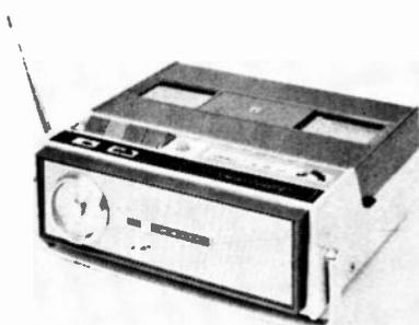
recorder features push-button operation; fast forward; automatic level operation; a.c. bias recording with 100 to 10,000 Hz response; 1 W output; 2-speed capstan drive; dual-track, 2-head recorder; vu meter; tape speed 3 3/4 & 1 1/4 ips; comes complete with dynamic mic; telephone pickup; patch cord, monitoring earphone, tape & take-up reel & batteries. Optional a.c. adapter available, 11 1/2" x 5" x 10 1/4". .....\$109.95
