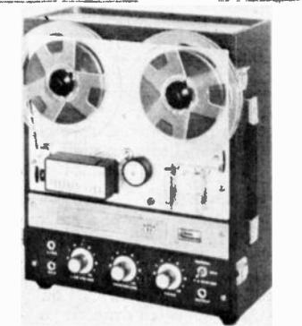
meter; counter; response 40-12,000 Hz ±3 dB @ 7½ ips; S/N ratio 45 dB; wow & flutter 0.2% @ 7½ ips; record/play & erase heads; 3 W peak output; vacuum-tube design; 4" x 6" spkrs. 15½ x 13½" x 7½" d. Supplied with dynamic mic .....\$179.95
