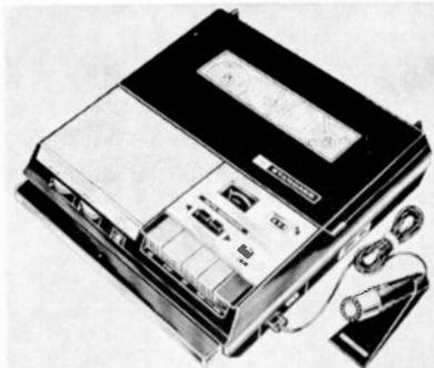
erate from 117 V or 230 V, 50/60 Hz or from 12 V d.c. (8 "D" cells). Transistorized design has automatic record level position & monitor facilities; record level & battery life indicator; 3-digit counter; 5" reels. Will replay tape in either direction plus endless play. Response 100-7000 Hz  $\pm$  5 dB @ 3 3/4 ips. Power 1.5 W max; S/N ratio 40 dB @ 1 kHz. Supplied with dynamic mic with remote control switch, power cord. 11 1/16" x 11 3/16" x 3 3/8" ....\$139.95
