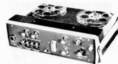
Hz. Three speeds (7 1/2, 3 3/4 & 1 7/8 ips); electronic speed control; maximum reel diameter 7", with cover 5". Response 40-16,000 Hz @ 7 1/2 ips; S/N ratio 56 dB at maximum recording level @ 7 1/2 ips; wow
