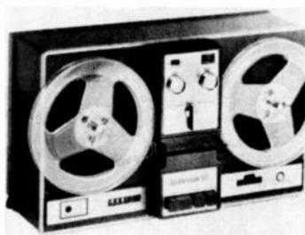
vu meter; pause control; counter; automatic shut-off; monitor facility; automatic head demagnetization. Response 40-17,000 Hz  $\pm 3$  dB @ 7½ ips; wow & flutter 0.25% @ 7½ ips; S/N ratio 48 dB @ 7½ ips; output 3 W dynamic power at 5% HD. Has mic & phono/radio inputs. 16" w. x 10" x 7" d. Supplied with protective cover & mic. ....\$159.95
