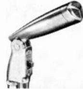
Dynamic; omnidirectional; frequency response 60 to 12,000 Hz; output —56 dB; high and low impedance; cast case; hinge head; on-off switch; built-in MC-4 connector ¼"-27 thread; satin chrome; 15 foot cable; size 7½" x 1¼"; weight 15 oz. ....\$57.00
