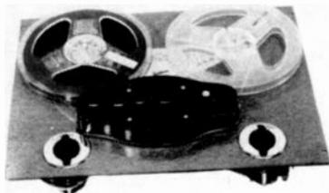
3 speeds; 3 motors; frequency response: 3.75 ips, 50 to 6000 Hz; 7.5 ips, 50 to 12,000 Hz; 15 ips, 30 to 15,000 Hz (all ±3 dB); flutter and wow less than 0.2%; tuning eye level indicator; dual track operation for up to 7" reel; requires preamp and amplifier; speed change by screw-on 2:1 ratio capstan sleeve and slow-fast stepped flywheel and motor pulley assembly; Mumetal heads; mechanical brakes;
