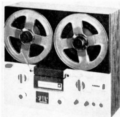
record/play); pause/cue control; dual-type vu meter. Response 50-15,000 Hz @ 7 $\frac{1}{2}$  ips; wow & flutter 0.15% @ 7 $\frac{1}{2}$  ips; S, N ratio 50 dB @ 7 $\frac{1}{2}$  ips. Features sound-with-sound & automatic shut-off. Accepts up to 7" reels. Does not have power amps. Has two line & two mic inputs & two line outputs, 14 $\frac{1}{2}$ " w. x 19" x 4 $\frac{1}{2}$ " .....\$169.95
