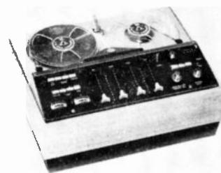
with built-in power amplifiers; three inputs (200-ohm mic, RIAA equalized phono, radio tuner) mixed via professional-type slide potentiometers; provision for sound-on-sound and echo; two record-level meters; hysteresis synchronous motor; separate record and playback heads; tape-input monitoring; preamp output; all plug-in circuit boards; 40-16,000 Hz  $\pm 2$  dB; r.m.s. flutter less than 0.075%; peak-to-peak flutter less than 0.2%; S/N ratio 50 dB. ....\$498.00
