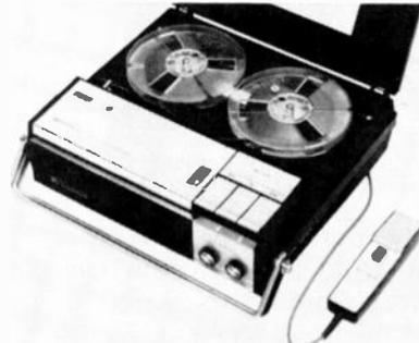
in a.c. converter for 117 V operation. Features automatic record level control; aux. high-level input; counter; record monitoring through speaker; can be used for p.a. Response 50-13,000 Hz @ 3¼ ips; wow & flutter 0.15% @ 3¼ ips; S/N ratio 48 dB. Supplied with remote-control Sony
