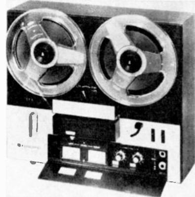
has two vu meters; 7" reels; automatic shut-off; cue control; counter. Response 30-18,000 Hz  $\pm$ 3 dB @ 7 $\frac{1}{2}$  ips (30-10,000 Hz @ 3 $\frac{3}{4}$  ips) wow & flutter 0.17%; S, N ratio 50 dB. Mahogany cabinet, 14 $\frac{3}{4}$ " x 12 $\frac{1}{2}$ " x 4 $\frac{1}{4}$ " .....under \$150.00
