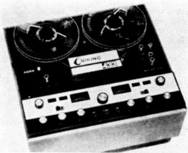
design; response 40-18,000 Hz  $\pm 3$  dB @ 7½ ips; S/N ratio 54 dB; THD 1% at 0 level; flutter & wow 0.2% @ 7½ ips; inputs for 0 level: mic 0.5 mV; aux. 75 mV. Features solid-state design; 3 heads; mixing controls; echo sw.; sound-with and sound-on-sound; counter; pause control; automatic shut-off. Has preamps only; output 1 V low impedance. 15¼" x 14¾" x 6½" behind panel .....\$369.95
