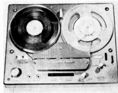
control. Tape speed 7 1/2, 3 3/4 & 1 7/8 ips. Has preamps only. Mono center channel output 1 V @ 200 ohms & dual stereo outputs 1.5 V @ 2000 ohms & 150 mV @ 10,000 ohms. Oscillator is transistorized, balance tubes. Dist. 0.5% at max. record level & 0.2% at max. playback level. Response at 7 1/2 ips is 30-20,000 Hz  $\pm$  2 dB; wow 0.1%; S/N 62 dB. 15 3/8" x 11 3/16" x 6 13/16". Has teak wood cabinet. Model 64X Four-track .....\$549.00
