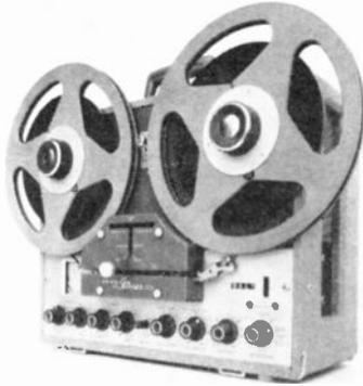
mic & line inputs with individual control knobs; sound-on-sound; 3 heads (record, playback, erase); bias indicator lights. Monitor before recording or off the tape; 2-speed (7 1/2 & 3 3/4 ips); 4-digit counter; automatic shutoff. Response 30-18,000 Hz  $\pm$  2 dB @ 7 1/2 ips; wow & flutter .15% @ 7 1/2 ips; S/N 55 dB; HD 1%; output 5 V from cathode followers. Size unmounted 12 1/8" x 16" x 8".
