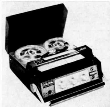
record head system. Response 40-20,000 Hz ±2 dB @ 7½ ips; S/N -45 dB; wow & flutter .18% @ 7½ ips; 4 W/ch output. Features 3 heads; ¼-track record & play; 17 hours recording time @ 1516 ips; 5" reel; 4 tracks; 6 V rechargeable battery (120 V
