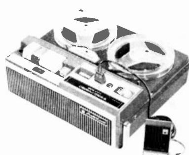
plug in; push button operation with fast forward; automatic level control, a.c. bias for 100-10,000 Hz record/playback; vu meter; 4 hours recording time @ 1 1/4 ips & 0.5-mil tape, 2 hours @ 3 3/4 ips; comes complete with dynamic mic with remote control sw.; telephone pickup, input patch cord, monitoring earphone, batteries, tape & 5" take-up reel; charcoal & grey with red & chrome trim; has 3" x 5" speaker, 10 1/2" x 4 1/2" x 8 1/2"; 6.7 lbs., .....\$74.95
