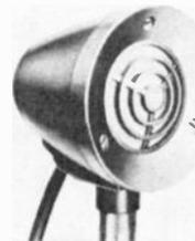
phragm is impervious to moisture and rain; response 60-10,000 Hz; output level -55 dBm (EIA rating, -150 dB); can be used with amplifiers having 150-250 ohm input; 15 oz.; supplied with 25' two-conductor cable. ....\$23.40
