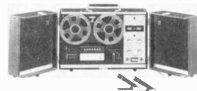
counter, 2 dynamic mics, cue button, monitor, sound-with-sound. Has mic & high-Z inputs; "Trans-A-Track" recording facility. Model 727 2-speed (7 1/2 & 3 3/4 ips); one ea erase & record/playback heads; unidirectional tape transport; response 30-20,000 Hz ±3 dB; wow & flutter 0.15% @ 7 1/2 ips; S/N ratio 50 dB; 6" speakers; 7 1/2 W/ch output; automatic shut-off. Mahogany ....\$300.00
