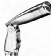
Dynamic; omnidirectional; frequency response 60 to 12,000 Hz; output —56 dB; high and low impedance; cast case; hinge head; on-off switch; built-in MC-4 connector ¼"-27 thread; satin chrome; 15 foot cable; size 7½" x 1¼"; weight 15 oz. ....\$57.00
