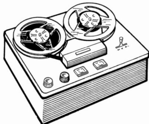
*The tape deck will record and play back and may have a separate playback head that permits off-the-tape monitoring. Neither power amplifiers nor speakers are included.*
