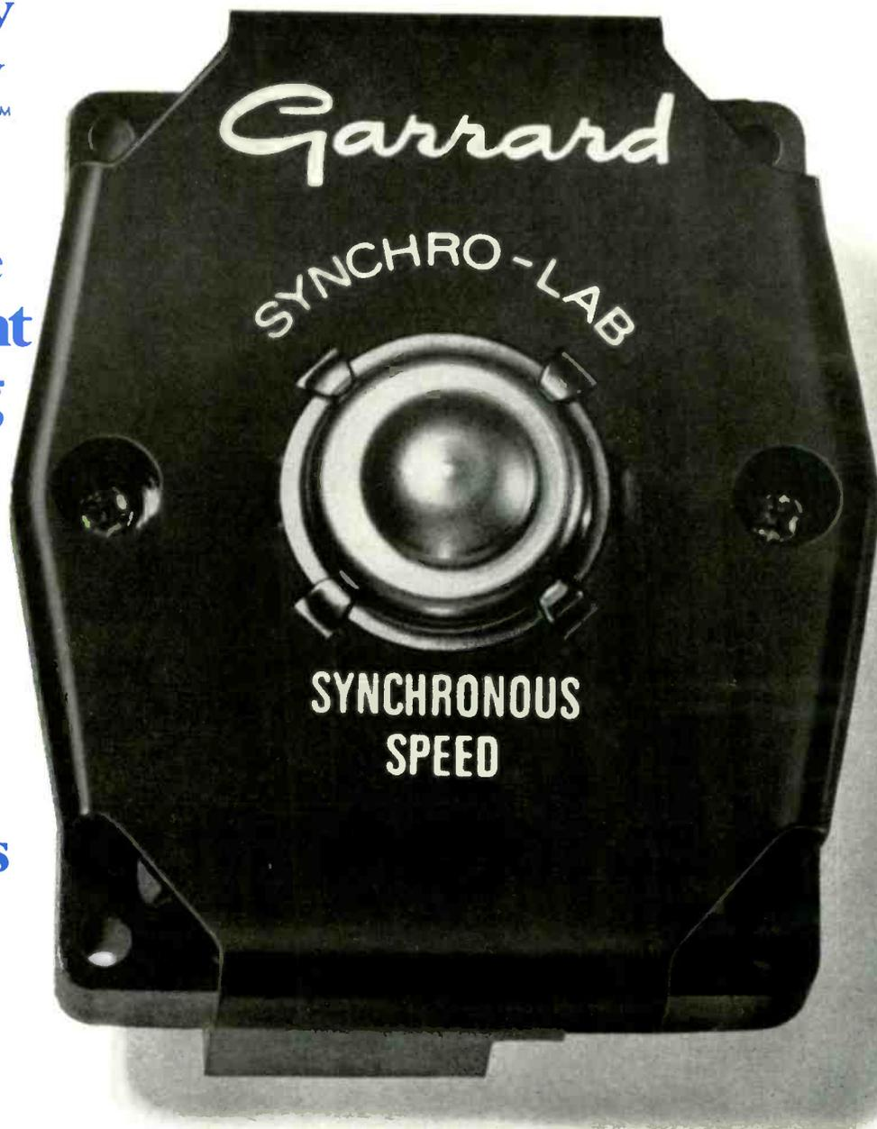
The ingenious new Synchro-Lab Motor incorporates the best features of both induction and synchronous motors: instant, full-power start and constant speed regardless of variations in voltage, temperature, stylus pressure or turntable load. It accomplishes this by "locking in" to the 60 cycle line current. It cannot fluctuate. The Synchro-Lab Motor also provides dependable driving torque and exceptional freedom from rumble.
