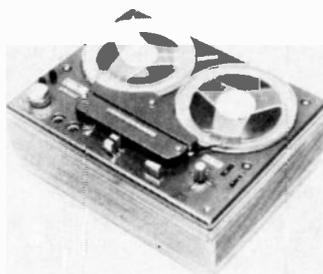
and record/playback heads; 2 level indicators; center-channel output; two 4" x 7" built-in speakers. Power output 3 W max for int. speakers & 10 W max continuous power (5% HD) for remote speakers. Response 40-16,000 Hz  $\pm$  2 dB @ 7 1/2 ips; inputs: low-Z mic 0.15 mV sensitivity; high level, 1 megohm, 75 mV sensitivity; low level, 100,000 ohms, 7.5 mV sensitivity. 15 3/8" x 11 3/16" x 6 7/8". Teak cabinet and TC-57B carrying case .....\$498.00
