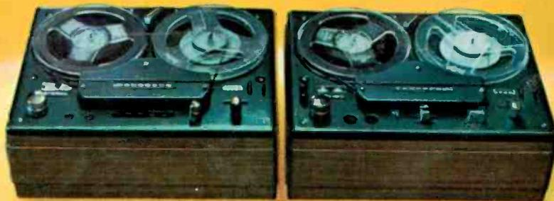
TANDBERG MODEL 54X (left) four-track stereo tape deck has three tape speeds and four separate tape heads for record, playback, erase and bias. FM stereo multiplex recordings are obtained with unparalleled brilliance. It features maximum versatility through built-in facilities for sound-on-sound, echo effects, add-a-track, direct monitor and remote control. \$549.
