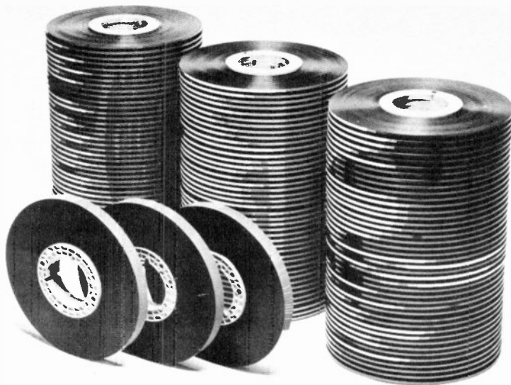
As the tape is slit, it is wound onto hubs. These rolls of tape are known as pancakes.
