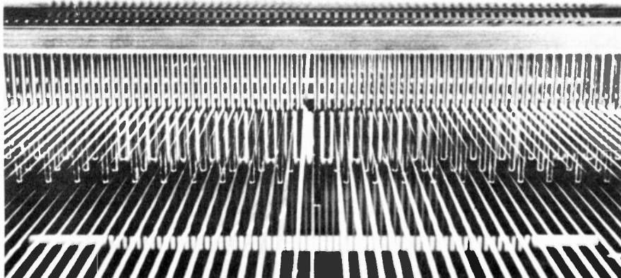
Recording tape is coated in broad rolls, then slit into appropriate widths on machines like this one.
