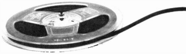
Open-reel tape is wound in a pancake shape on a plastic reel similar to home movie-film reel.
