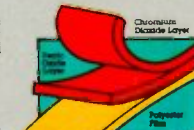
Two distinct and different oxide layers for "extra loud" playback in car stereo systems.
