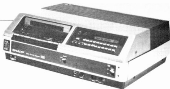
Microprocessor-controlled Sharp VC-6700 can fast-wind to any tape location programmed on its 10-key pad.
