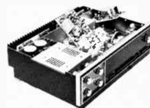
Hinged circuit boards for FM IF, AM IF, Multiplex and Phono Preamp sections — six plug-in boards for all other major circuitry.
