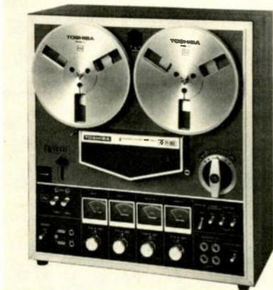
speeds (1 7/8, 3 3/4 & 7 1/2 ips), 3 heads. Response 30-20,000 Hz ±3 dB with low-noise tape. (S+N)/N 50 dB. Wow & flutter 0.09% at 7 1/2 ips. Has regular & low-noise tape switch. 15 3/4" x 17 1/2" H x 8 3/4" D. . . . . \$499.95
