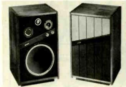
20-25,000 Hz; 8 ohms imp.; crossovers 1000 & 5000 Hz; 180-degree dispersion; front-panel mid-range & tweeter controls; removable two-tone double-knit acoustic grille; hardwood walnut veneer on wood products; max. power 90 W; min. power 10 W. 31" H (inc. base) x 18 3/4" W x 15 3/4" D..... \$239.00
