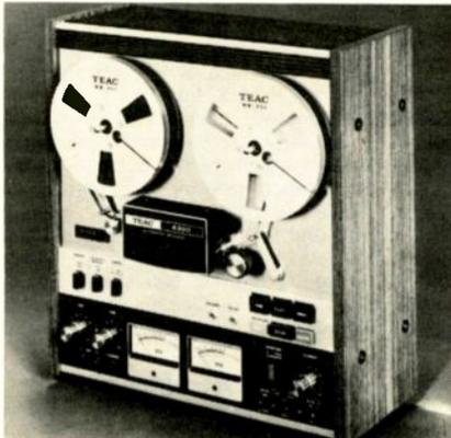
transport control, pause control with indicator light, dual VU meters; separate bias/equalization switches; separate mike/line inputs; separate mike/line level controls. Will handle up to 7" reels. Includes memory counter for automatic repeat and memory marker level guides; total remote-control capability. Response 40-24,000 Hz; wow & flutter 0.06% both at 7 1/2 ips. S/N 65 dB (WTD at 3% THD). 17 3/16" x 19 1/4" x 8 1/2" ..... \$699.50
