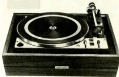
angle selector for single- and multiple-play. Tracking down to  $\frac{1}{2}$  gram. Damped counterbalance with coarse and fine adjustments. Synchronous/hi-torque motor, 4-lb one-piece die-cast platter; illuminated strobe. 13" x 10 $\frac{3}{4}$ " plus 1" at rear and right for tonearm overhang. 5" above and 2 $\frac{3}{4}$ " below mounting board. .... \$199.95
