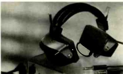
realistic spatial distribution of sound; two dynamic drivers per phone; response 20-20,000 Hz; sensitivity 100 dB SPL at 1000 Hz for 1 mW; dist. 0.2% max; features "Quadrablend"
