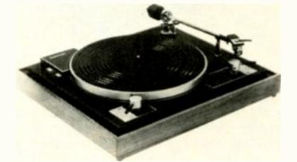
up assembly. Has push-button speed control; hydraulic lift and lowering of tonearm; anti-vibration springs; lightweight cartridge shell with self-cleaning contacts. Two-speed (33 & 45 rpm); 60-Hz synchronous constant speed 450 rpm; belt drive. Rumble -50 dB (RIAA); hum -80 dB; wow & flutter 0.1%. Has 10 $\frac{1}{4}$ " aluminum platter. 13 $\frac{3}{4}$ " x 15 $\frac{1}{2}$ " x 4 $\frac{1}{2}$ " H (including dust cover). Comes with arm, base, dust cover but without cartridge. .... \$144.95
