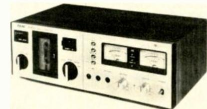
rotary lever transport-control system; separate bias/equalization switches; LED peak indicator; response 30-16,000 Hz (CrO<sub>2</sub> tape), S/N 60 dB (WTD with Dolby); wow & flutter 0.08%. . . . . \$329.50
