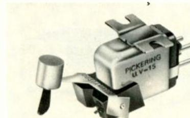
load and 100 pF); output 3.3 mV  $\pm$  2 dB; channel separation 35 dB; inductance each channel 350 mH; resistance each channel 750 ohms; comes with "Quadrangular" diamond stylus assembly. . . . . \$125.00
