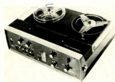
Portable (15 V, ten 1 1/2-V cells), mono design. Three speeds (7 1/2, 3 3/4, 1 7/8 ips), and has three heads. Will handle up to 7" reels. Has automatic level-input controls, mike & line mixing, and built-in speaker. Response 40-16,000 Hz  $\pm 2$  dB at 7 1/2 ips, wow 0.1% at 7 1/2 ips, (S + N)/N 58 dB unweighted. 13" W x 10" D x 4".
