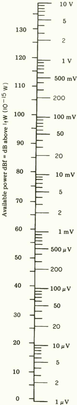
$E_0 = \text{Open-circuit input voltage} - 300 \Omega \text{ source}$
