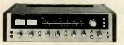
47 W rms/ch into 8 ohms at 0.5% THD (20-20,000 Hz) with both channels driven; power bandwidth 12-50,000 Hz; input sensitivity: mag. phono #2 150 mV (low), 40 mV (high), aux. 250 mV, tape A & B 500 mV, mike 6 mV; hum & noise: mag. -68 dB, aux. -75 dB; FM sensitivity 1.65  $\mu$ V; capture ratio 1.5 dB; stereo separation 40 dB; has FM and audio muting, main/remote speaker outputs. 19 $\frac{1}{8}$ " W  $\times$  5 $\frac{1}{2}$ " H  $\times$  14 $\frac{1}{4}$ " D. . . . . \$399.95
