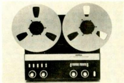
10 1/2" reels. Response 30-20,000 Hz  $\pm$  2.5 dB at 7 1/2 ips. Wow & flutter 0.08% peak at 7 1/2 ips. (S + N)/N 61 dB at 7 1/2 ips. Has a servo braking system, VU meters, automatic shut-off, relay and solenoid operation, full remote control, and off-the-tape monitoring. Options include plug-in power amplifiers, a suitcase version with built-in speakers, metal cage for rack or custom mounting. 16 3/8" H  $\times$  14 1/8" W  $\times$  7 1/8" D ..... \$959.00
