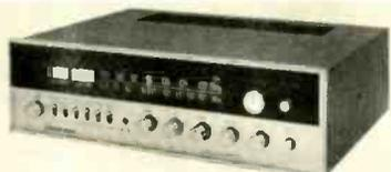
rejection 53 dB; i.f. rejection 85 dB; capture ratio 1.5 dB; S/N 65 dB; HD 0.5%; stereo separation 37 dB; selectivity 46 dB. Features fine-
