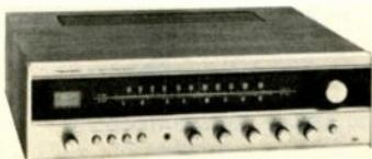
$\mu$ V; capture ratio 3 dB; image rejection 50 dB; alternate channel rejection 50 dB; THD 1% 1 mV mono; S/N 65 dB 1 mV; stereo separation 34 dB at 1000 Hz; features FM muting; regulated power supply; "Quatravox" for synthesizing 4-channel by adding second set of speakers; has tape monitor; headphone jack; main/remote speaker switch; 75 & 300 ohm FM antenna inputs; blackout dial. Wood cabinet. 5 $\frac{1}{4}$ " x 18 $\frac{3}{4}$ " x 13 $\frac{1}{2}$ " ..... \$249.95
