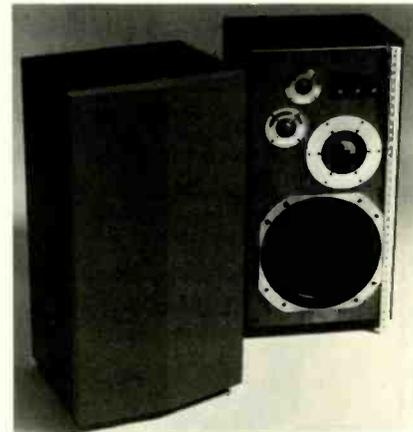
frequency driver (4000-8000 Hz), 3/4" super tweeter (8000-35,000 Hz); new diaphragm material strong enough to withstand 93-g accelerations; baffle board of beech lumber-core laminated with crosswise and lengthwise oak veneer; will handle 150 W; efficiency 94 dB; imp. 8 ohms; dist. 0.5% dispersion 30 degrees 0 dB, 60 degrees -3 dB. 18 1/2" W x 37" H x 15" D..... \$1350.00
