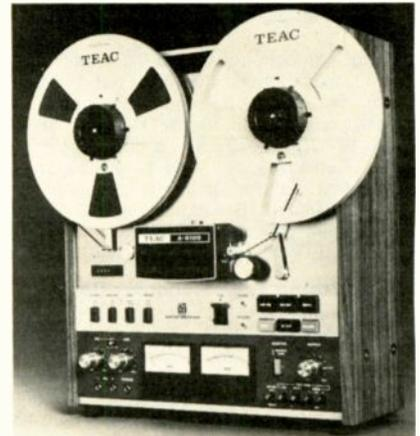
Two-speed (15 & 7½ ips), two-track, two-channel stereo with four heads (erase, record, playback, 4-track playback); 3 motors. Will handle 10½" & 7" reels. Features cue button & flip-up head cover for easy editing; auto stop counter; mike attenuation control; LED peak level indicators. Response 30-26,000 Hz at 15 ips; wow & flutter 0.04% at 15 ips; S/N 67 dB (WTD at 3% THD). 17⅞" W x 20⅞" H x 8⅞" D. .... \$1049.50
