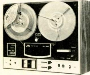
7½ ips; (S + N)/N -52 dB; wow & flutter 0.13% rms at 7½ ips. Has mike (0.5 mV) & aux. (80 mV) inputs. Line output 0-1 V. Has switch for either low-noise or standard tape; two heads (record/play and erase). 7½" × 15¾" W × 12¾" D. . . . . \$249.95
