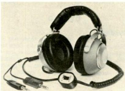
(blue for front, black for rear); earpieces marked "L" and "R" for accurate listening orientation. Sensitivity: 100 dB SPL (at 0.1 V input at 1 kHz each channel). Maximum power input 1.25 V rms continuous with provision for 10 dB SPL transient peaks. Dist. 1/2% at 110 dB SPL. Input imp. (at 1 kHz) 15 ohms ±20%. Vinyl-covered foam ear cushions; adjustable headband. 11-ft coiled cord with four-channel/stereo switch, front & rear plugs. 19 ounces. . . . . \$69.95
