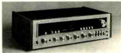
jection circuit; triple tone controls. FM sensitivity 1.7  $\mu$ V; quieting slope 56 dB at 5  $\mu$ V; S/N 72 dB; capture ratio 1.3 dB; alternate channel selectivity 80 dB; stereo separation 45 dB at 1000 Hz, 35 dB at 10,000 Hz; HD 0.5% stereo (400 Hz, 100% mod.); image rejection 80 dB; spurious rejection 90 dB; multi-path detection meter; deviation meter. 21 $\frac{9}{16}$ " W  $\times$  6 $\frac{1}{16}$ " H  $\times$  15 $\frac{1}{16}$ " D. . . . . \$749.95
