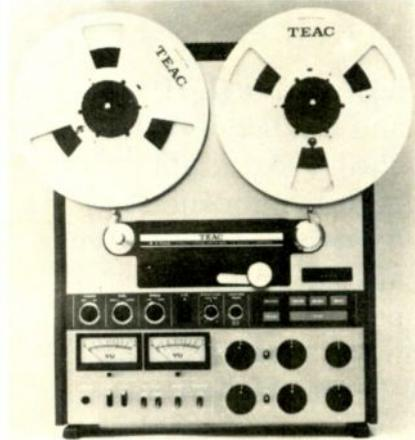
stan/servo control motor; two a.c. reel motors; built-in mixer to blend up to 4 mikes or lines; separate master input level control for all mike/line inputs; separate output level control. Has two sets of output jacks; dual VU meters; 3-position bias/equalization switches; pitch control; cue facility; push-button transport control; logic circuitry. Response 40-24,000 Hz; wow & flutter 0.05%, both at 7 1/2 ips. S/N 65 dB (WTD at 3% THD). . . . . \$1399.50
