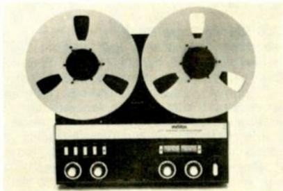
10 1/2" reels. Response 30-20,000 Hz  $\pm 2.5$  dB at 7 1/2 ips. Wow & flutter 0.08% peak at 7 1/2 ips. (S + N)/N 61 dB at 7 1/2 ips. Has a servo braking system, VU meters, automatic shut-off, relay and solenoid operation, full remote control, and off-the-tape monitoring. Options include plug-in power amplifiers, a suitcase version with built-in speakers, metal cage for rack or custom mounting. 16 3/8" H x 14 1/8" W x 7 1/8" D ..... \$959.00
