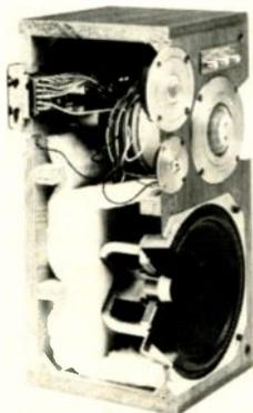
system; 12" woofer, 2 1/2" dome mid-range, 1" dome tweeter, 5/8" dome super tweeter; response 30-35,000 Hz; crossovers: ferrite core inductors 600, 5000, 10,000 Hz; metalized polyester film capacitors above 10,000 Hz; imp. 6 ohms; output acoustic pressure 90 dB/W at 1 meter; will handle 100 W peak. 14 1/4" W x 24 1/2" H x 13" D. . . . . \$580.00
