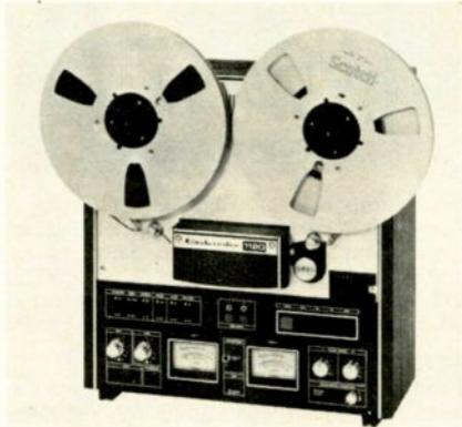
2-channel deck or can be converted to a 2-track, 2-channel record/play deck; provides built-in circuitry for synthetic echo, sound-on-sound, sound-with-sound, and locking pause control for editing tape while recording or during playback. Wow & flutter 0.06%, S/N 60 dB, crosstalk 58 dB at 1 kHz, response 25-24,000 Hz, all at 7½ ips. 16¾" W × 17¾" H × 6¾" D. . . . . \$649.95
