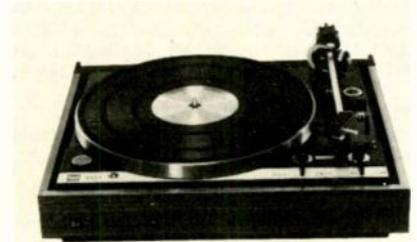
plus rotor) 9.7 lbs. Gimbal-mounted 8 $\frac{3}{4}$ " tonearm. Two anti-resonance filters integral with counterbalance, tuned to tonearm/cartridge system and chassis. Stylus pressure 0-3.0 g, calibrated in 10ths of a gram. Anti-skating. Cueing system damped in both directions. Rumble: -70 dB. Wow & flutter: 0.03%. 16.5" x 14.4" x 5.8". With base and dust cover ..... \$400.00
