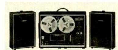
& 1 7/8 ips), straight-line record & playback level controls, two VU meters, automatic end-of-tape shutoff, and sound-on-sound. 5 W/ch continuous power. Response 30-18,000 Hz  $\pm 3$  dB at 7 1/2 ips. (S + N)/N 50 dB; wow & flutter 0.12% at 7 1/2 ips. Sensitivity: aux. 0.06 V; low-imp. mike -72 dB (can be used as phono input with optional RK-66 adapter). Has line output 0.43 V at 0 VU; two lid speakers. 8 ohms. 20 1/4" W x 10 1/4" H x 15 1/4" D. Comes with carrying case. \$399.95
