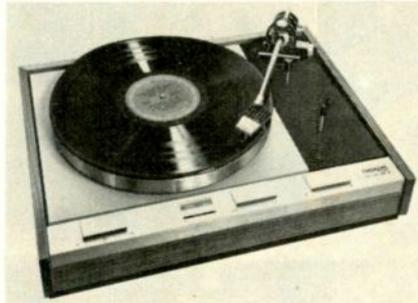
adjustment ±2%; illuminated strobe speed control; 12" non-magnetic zinc alloy platter; wow & flutter 0.06% weighted; rumble -45 dB (unweighted), -68 dB (weighted); features magnetic anti-skating control; isolated tonearm & drive system; cueing control. Comes with walnut base and TP-16 9.06" tonearm. 18" x 5" H x 14" W (with 9" tonearm) x 16" (with 12" tonearm) ..... \$410.00
