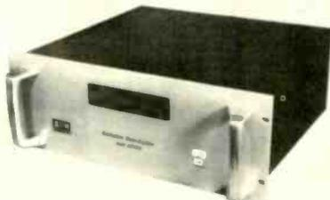
ohms at 0.2% THD; frequency response 2-75,000 Hz +0, -3 dB; 20-20,000 Hz +0, -0.2 dB; noise & hum 110 dB below rated output into 8 ohms; input sensitivity 2 V ±2% for 40 V out (200 W, 8 ohms); voltage gain 26 dB; damping factor 500; electronic power limiters; plug-in circuit modules. 19" rack mount × 7" H × 17" D ..... \$1499.00
