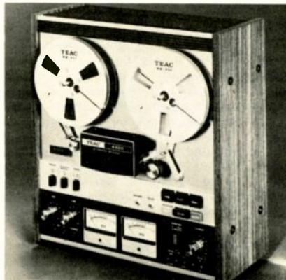
transport control, pause control with indicator light, dual VU meters; separate bias/equalization switches; separate mike/line inputs; separate mike/line level controls. Will handle up to 7" reels. Includes memory counter for automatic repeat and memory marker level guides; total remote-control capability. Response 40-24,000 Hz; wow & flutter 0.06% both at 7½ ips. S/N 65 dB (WTD at 3% THD). 17⅞" x 19¼" x 8½" ..... \$699.50
