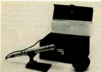
Dynamic unidirectional moving-coil type; cardioid pattern; response 40-18,000 Hz; impedance 600 ohms; comes with windscreen, clamp, table stand, and case; Cannon XLR connector; each unit supplied with own frequency-response curve. .... \$165.00
