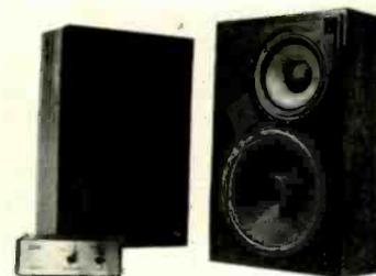
response 32-18,000 Hz ±3 dB, below 40 Hz, down 3 dB at tuning point of 32 Hz (sixth-order Butterworth); includes equalizer which adds mild boost of 6 dB at 35 Hz; below usable range of system equalizer rolls off electrical
