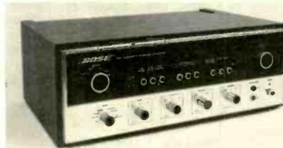
preamplification; low-noise phono preamp circuitry; modular PC board construction; tape recording flexibility; provision for external equalizers; compatibility with all types of program sources, modes, and equipment. 6" H × 18" W × 13 1/8" D ..... \$599.00
