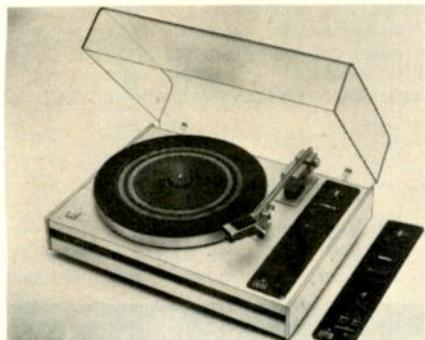
(turntable drive, pickup arm movement, cueing); separate fine-speed adjustment ±3%; wow & flutter 0.07%; rumble -43 dB (DIN A); stylus force 0.75-3 g adjustable; anti-skating force adjustable for spherical & elliptical styli; turntable drive 9 V d.c. motor with 72-pole tachogenerator; pickup arm lift touch-controlled, viscosity damped pickup arm lift; optional manual operation; photoelectric end-of-record switch-off system. 6 1/2" H x 17 1/8" W x 12 3/4" D ..... \$299.50
