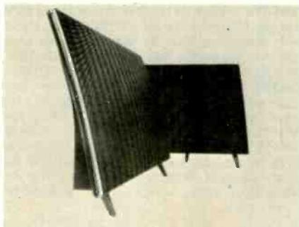
50-10,000 Hz, 100 dB 70-7000 Hz; bandwidth 45-18,000 Hz; attenuation 18 dB/octave; dispersion 70 degrees horizontal, 15 degrees vertical; impedance 30-15 ohms (40-8000 Hz) falling above 8000 Hz; 100-120 V, 200-250 V, 50-60 Hz; front grille aluminum anodized bronze or black, polished wood end frames; 31" H x 34 1/2" W x 10 1/2" D. . . . . \$450.00
