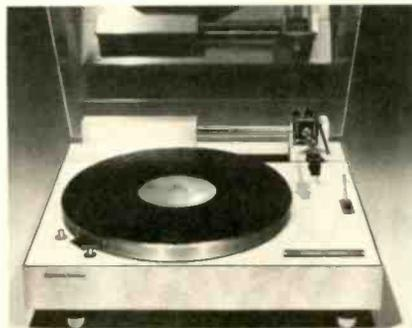
brushless d.c. (Hall Effect) motor with precision-ground belt; tracking error, skating force, vertical friction, lateral friction all 0; rumble (DIN B) -68 dB; wow & flutter (NAB weighted) 0.04%; (DIN B) 0.09%; hum -76 dB; speed constancy  $\pm 0.3\%$ ; viscous-damped cueing control; tonearm mass 6 gr.; comes with straight-line tracking arm; dust cover. 6 $\frac{3}{4}$ " H (with dust cover) x 16 $\frac{1}{2}$ " W x 16 $\frac{1}{4}$ " D. .... \$400.00
