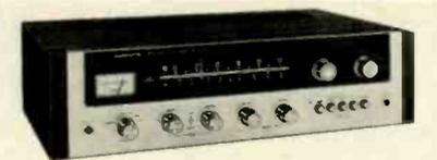
22 W rms/ch into 8 ohms at 0.5% THD (20-20,000 Hz) with both channels driven; power bandwidth 15-30,000 Hz; input sensitivity: mag. phono #2 6 mV (low), 2.5 mV (high), aux. 250 mV, tape 500 mV; hum & noise: aux. -75 dB, mag. phono -65 dB; FM sensitivity 1.75  $\mu$ V; capture ratio 1.5 dB; main/remote speaker switching; tape monitor; FM muting; front-panel stereo tape & headphone output. 17 $\frac{1}{16}$ " W  $\times$  5" H  $\times$  14" D. . . . . \$249.95
