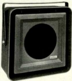
4000 Hz crossover; response 80-10,000 Hz; power handling 60 W peak; 8 ohms imp.; 120-degree dispersion; compression-molded glass-filled polyester enclosure; water-proof & fungus-proof, 21 1/2" H x 21 1/2" W x 8 1/2" D . . . . . \$109.50
