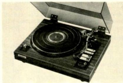
drive turntable with brushless d.c. servo motor; electronic speed change; speed control range ±2%; wow & flutter 0.05% W rms; S/N 60 dB; 12 1/4" aluminum alloy die-cast platter; static-balance S-shaped pipe tonearm; usable cartridge weight 4 to 32 g; anti-skating; oil-damped cueing device; stylus pressure direct-readout counterweight; lateral balancer; arm height adjustment; plug-in headshell. 18 7/8" W x 7 1/8" H x 16 3/8" D ..... \$299.95
