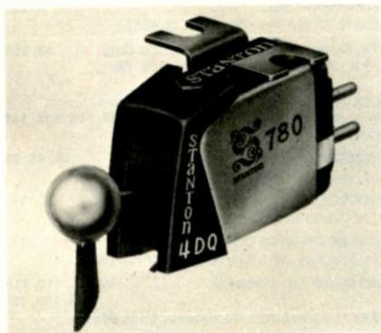
matrix-derived compatible records. Response 10-50,000 Hz (when terminated in recommended load of 100 kohms and 100 pF). Tracking force 1-3 g; channel separation 35 dB. Output: 0.7 mV/cm/sec ±2 dB. Inductance & resistance (each channel): 350 mH; 750 ohms. Features new "Quadraredral" stylus ..... \$125.00
