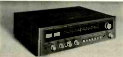
$\pm$ 1 dB; FM sensitivity 1.8  $\mu$ V (IHF); capture ratio 1.5 dB; image rejection 70 dB; S/N 70 dB; HD 0.7% stereo; features signal-strength and center-tuning meters; separable left & right tone controls; outputs for three speaker systems; tape-to-tape dubbing facilities; full complement of input and output terminals, jacks, switches, and terminals. Walnut-grained vinyl over Luan plywood. 18 1/2" W x 14 3/4" D x 5 1/2" H. \$449.95
