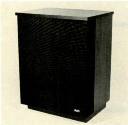
with 3" cone, 1" dome tweeter, two side-firing 1½" auxiliary tweeters; crossovers at 500 Hz, 4000 Hz, 9000 Hz. Will handle 200 W program power; 25 W min. recommended. 8 ohm imp. Frequency response 30-18,000 Hz ±2 dB. Separate 3-position mid-range & high-frequency level switches; fuse-overload protection. Brown grille cloth; top optional in black high-pressure laminate or walnut; walnut sides. 26½" H × 20½" W × 15" D. 5-year transferable warranty. . . . . \$300.00
