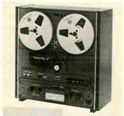
and 2 six-pole eddy-current type induction motors; automatic tape lifters; automatic shut-off; tape selector switch; echo & sound-on-sound; tape/source monitor. Wow & flutter 0.08% W rms at 7½ ips. (S + N)/N 55 dB. Response 40-21,000 Hz at 7½ ips . . . . . \$399.95
