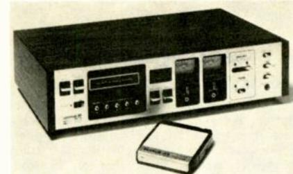
3M ferric-oxide tape. Has minutes/seconds timer for precise timing of recordings; fast-forward mode 3 1/2 times actual speed; special cueing system. Response 30-15,000 Hz ±3 dB with Scotch special high-performance tape (30-12,000 Hz with standard tape). (S + N)/N 60 dB at 4000 Hz and above (Dolby system on). Sensitivity: mike 0.25 mV; aux. 80 mV. 19 3/4" x 5" x 10 1/4" . . . . . \$399.95
