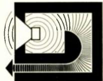
VENTURI cabinet is the terminus of the Venturi path inside the enclosure (U.S. Pat. 3892288). It works as an acoustic transformer to produce bass energy as much as 140 times greater than would otherwise be achievable from a woofer alone in the same size cabinet.
