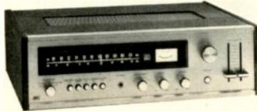
30-20,000 Hz  $\pm$ 1 dB; S/N 60 dB (phono), 80 dB (aux.); FM sensitivity 2.5  $\mu$ V (IHF); capture ratio 2 dB; stereo separation 35 dB at 1000 Hz; features "Auto-Magic" tuning system which fine-tunes station electronically; "Perfect Loudness" slide controls for volume and balance settings; "Quatravox" 4-ch synthesizer; FM muting; tape monitor; high filter; main/remote speaker switching; headphone jack. Walnut veneer cabinet. 5" x 17 $\frac{1}{8}$ " x 12 $\frac{1}{2}$ " ..... \$299.95
