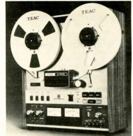
Two-speed (15 & 7 1/2 ips), two-track, two-channel stereo with four heads (erase, record, playback, 4-track playback); 3 motors. Will handle 10 1/2" & 7" reels. Features cue button & flip-up head cover for easy editing; auto stop counter; mike attenuation control; LED peak level indicators. Response 30-26,000 Hz at 15 ips; wow & flutter 0.04% at 15 ips; S/N 67 dB (WTD at 3% THD). 17 3/8" W x 20 1/2" H x 8 1/4" D. .... \$1049.50
