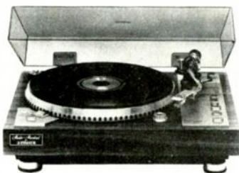
of manual start/stop; quartz PLL speed control, ±6% range unlocked; S-shaped balanced tonearm; viscous damped cueing and variable anti-skate; strobe light and pitch control; adjustable legs, integrated level and stylus overhang gauge; wow and flutter 0.03% wrms; rumble -70 dB (DIN "B"); tracking force range 0.6-3.5 g; tracking error ±1.5 degrees; 12 1/4-in platter; effective arm length 222 mm; cartridge mounting hardware; walnut base; 6 1/2" H x 17 1/4" W x 14 1/4" D..... \$300
