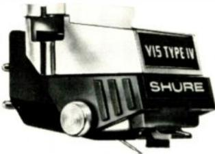
Hz; channel separation 25 dB at 1000 Hz; tracking force 0.75-1.25 g;  $0.2 \times 0.7$  mil biradial hyperelliptical stylus; features viscous damped dynamic stabilizer; replacement stylus VN45HE ..... \$150
