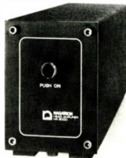
quency response 10-200,000 Hz  $\pm 1$  dB; 40-dB gain; THD 0.01% at 1000 Hz; noise level at input -155 dB/V (RIAA and IHF "A"); max. input 8.4 mV; output to magnetic phono in 50,000 ohms; input impedance 20 ohms; battery-powered with individual power supplies/channel ..... \$275
