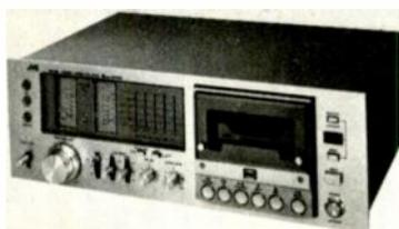
Front-loading stereo cassette deck with super ANRS noise-reduction system and recording equalizer circuit; independent drive motors: FG servo type for capstan, dc type for reel drive; two-head configuration: Sen-Alloy record/playback head, double-gap ferrite erase head; push-button full-logic solenoid operation; independent mic and line inputs; three-
