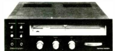
ture ratio 1.5 dB; S/N 64 dB; image response -100 dB; i-f response -100 dB; frequency response 10-50,000 Hz  $\pm$  0.5 dB; has FM quieting meter for tuning; two-stage muting system (wide and narrow); pushbutton for external processor use; 25  $\mu$ sec de-emphasis; noise filter; headphone monitoring; output level adjustment; 4 $\frac{1}{2}$ " H  $\times$  16" W  $\times$  13 $\frac{1}{2}$ " D ..... \$630
