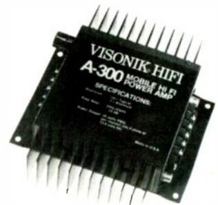
channels; oscillator-driven push-pull inverted circuit with ferrite-core power transformer; low-current remote turn-on feature; one-piece printed circuit board construction for all components and connectors; clamped power transistors to extruded heat sinks..... \$136
