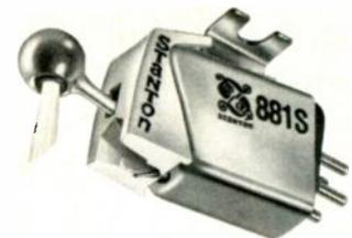
$\pm 1$  dB/35 dB; load impedance 47,000 ohms; load capacitance 275 pF (including arm leads, cables, and amp); tracking force 0.75-1.25 g; nude Stereohedron stylus; weight 5.7 g with self-supporting (1 g) brush; replacement stylus DB1, DB10 for mono LP's, DB27 for 7B's ..... \$150
