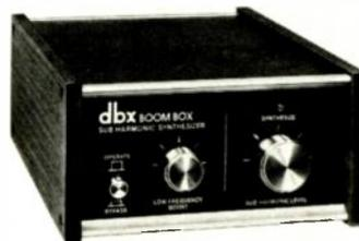
60 Hz to recreate signals in bottom octave; can be inserted in tape monitor circuit of receiver or amplifier; synthesizes and low-frequency boost controls plus bypass switch; input impedance 47,000 ohms; output level 7 V rms; frequency response 20-20,000 Hz  $\pm 1$  dB; THD 0.1%; 3 3/4" H x 7 1/4" W x 10 1/4" D..... \$199
