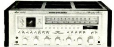
ohms at 0.05% THD; five-gang dual-gate MOS FET FM front end; quartz-lock FM tuning; PLL FM multiplex demodulator; full complementary direct coupled output; turbo-flow heat dissipation system; built-in 3-in oscilloscope display; peak indicators; plug-in Dolby FM capability; high- (9 kHz, 18 dB/octave) and low-frequency (15 Hz, 18 dB/octave) filters; independent tape-to-tape copy; 7" H x 19 $\frac{1}{4}$ " W x 17 $\frac{1}{8}$ " D..... \$1600
