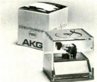
±1 dB/30 dB at 1 kHz; optimum load impedance 47,000 ohms; optimum load capacitance 470 pF; tracking force 0.75-1.25 g; 0.2 × 0.7 mil elliptical diamond stylus; supplied with frequency response/crosstalk curve and screwdriver; weight 5.86 g..... \$135
