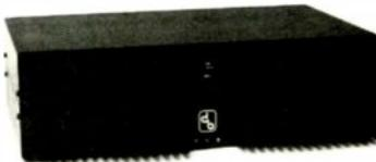
ance 1 V/50,000 ohms; S/N 113 dB at 1 V in (A weighted), 96 dB at 1 W into 8 ohms (A weighted); slew rate 15 V/ $\mu$ sec; damping factor greater than 400 from 20-1000 Hz, 40 at 20,000 Hz. Features 12 dB/octave subsonic filter; peak-clipping LEDs; electronic clamp (in place of relays). 4.9" H x 16" W x 12.8" D..... \$595
