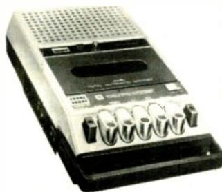
cue and review; chromium dioxide switch; three-digit tape counter; record level/battery meter; tone control; three-way power; auto shut-off; auto recording level control; pause control; 1/4-in headphone jack; wow and flutter less than 0.35%; frequency response 50-10,000 Hz (CrO<sub>2</sub> tape), 80-90,000 Hz (standard tape); 6 1/2" H x 11" W x 2 1/4" D ..... \$70
