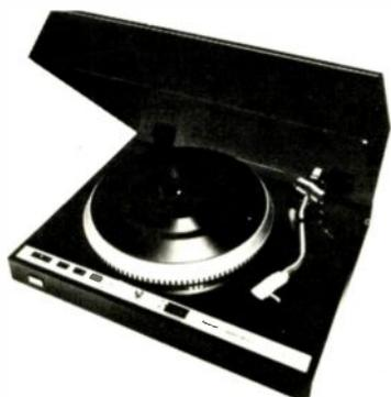
controls up front for convenience; oil-damped cueing; "S"-type arm with gold-plated headshell connector contacts; stroboscope; pitch control; quartz-lock defeat; wow and flutter 0.025%; speed deviation less than 0.002%; rumble below -72 dB; with base and removable, hinged dustcover; 6 $\frac{3}{8}$ " H  $\times$  19 $\frac{1}{8}$ " W  $\times$  15 $\frac{1}{8}$ " D . . . . . \$440
