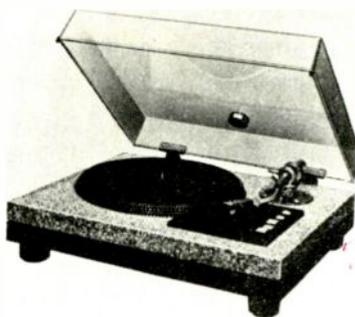
servomotor; granite composite motor board to resist acoustic feedback; audio-isolated legs; statically-balanced "S"-type tonearm with plug-in headshell, oil-damped cueing; anti-skating; micrometer-style counter-weight calibration; rosewood grained base; illuminated stroboscope; speed adjustment ±4%; wow and flutter less than 0.03% wrms; rumble less than -70 dB (DIN "B" weighting); tonearm effective length 9.6-in min. tracking force 1 g; 7.4" H x 19.8" W x 16.3" D..... \$300
