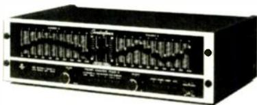
jacks; mono selector; reverse/stereo mode; four switched and two unswitched ac outlets. Specifications: frequency response 5-100,000 Hz  $\pm 0.25$  dB (high level), 20-20,000 Hz  $\pm 0.5$  dB (phono); THD and IM. dist. 0.05% at 1 V; gain 63 dB (phono), 21 dB (high level); output impedance 600 ohms max. Equalizer: S/N 96 dB; frequency response 10-100,000 Hz  $\pm 0.25$  dB. Silver/gold front panel in walnut side panels; 6" H  $\times$  19" W  $\times$  11" D ..... \$549
