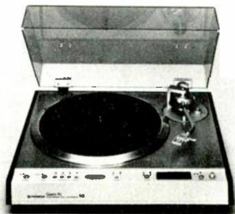
and meter display; optical-electronic end-of-play detection; electronic cueing device and quick-stop; anti-skating; S-curved gimbal-supported tonearm (effective length 237 mm); magnesium headshell; coaxial suspension system. Wow and flutter 0.025% wrms max.; rumble -65 dB (JIS), -75 dB (DIN "B"). Includes removable hinged acrylic cover. 5 3/8" H x 18 1/2" W x 16 7/8" D..... \$400
