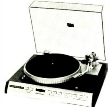
locked turntable with auto return/shutoff arm; dc servomotor; rpm speed/deviation digital readout; lateral balanced tonearm; oil-damped cueing; shock absorbent feet; anti-skating; wow and flutter 0.02% (NAB weighted); rumble -70 dB (NAB RRL); includes dustcover and walnut-finish base; 5<sup>3</sup>/<sub>8</sub>" H x 18<sup>1</sup>/<sub>4</sub>" W x 14<sup>1</sup>/<sub>2</sub>" D..... \$400
