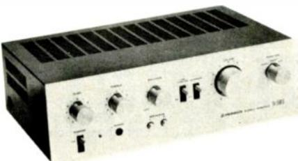
with 0.5% THD; IM dist. 0.5% at rated output; damping factor 30. Preamp section: input sensitivity/impedance 2.5 mV/50,000 ohms (phono), 150 mV/50,000 ohms (tuner, aux., tape); phono overload 130 mV (1 kHz); frequency response 20-20,000 Hz  $\pm 0.5$  dB (phono), 20-20,000 Hz  $\pm 1$  dB (tuner, aux., tape); hum and noise (IHF A) -71 dB (phono), -87 dB (tuner, aux., tape). 4<sup>7</sup>/<sub>16</sub>" H x 14<sup>3</sup>/<sub>32</sub>" W x 10<sup>1</sup>/<sub>32</sub>" D..... \$135
