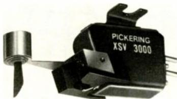
force 0.75-1.5 g; channel separation 35 dB; features Dustamatic brush; replacement stylus D3000 ..... \$100
