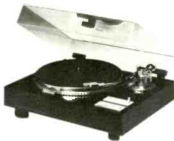
double FG/quartz PLL servo system with high-torque 12-pole, 24-slot dc servomotor; S-shaped arm on gimbal support; oil-damped cueing lever; direct-reading anti-skate device; acoustic insulator feet; stroboscopic speed indication on turntable rim
