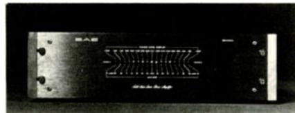
dist.; frequency response 20-20,000 Hz  $\pm 0.25$  dB; S/N 100 dB; input sensitivity 1.0 V. Features fully complementary circuits, toroid power supply, thermal, signal relay, and electronic protection, and LED display for output monitoring. 5 1/4" H  $\times$  19" W  $\times$  8 1/2" D ..... \$350
