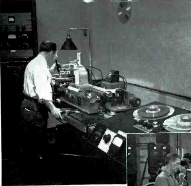
Above, the music is being transferred from tape to disc. Microscope at the operator's hand permits precise inspection of the record grooves. In the center illustration, a master
