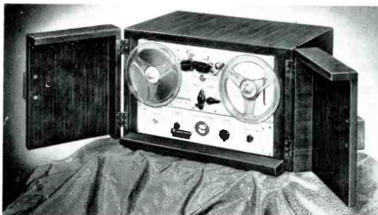
Fig. 2. The MagneCordette: tape mechanism with preamplifier, below.
