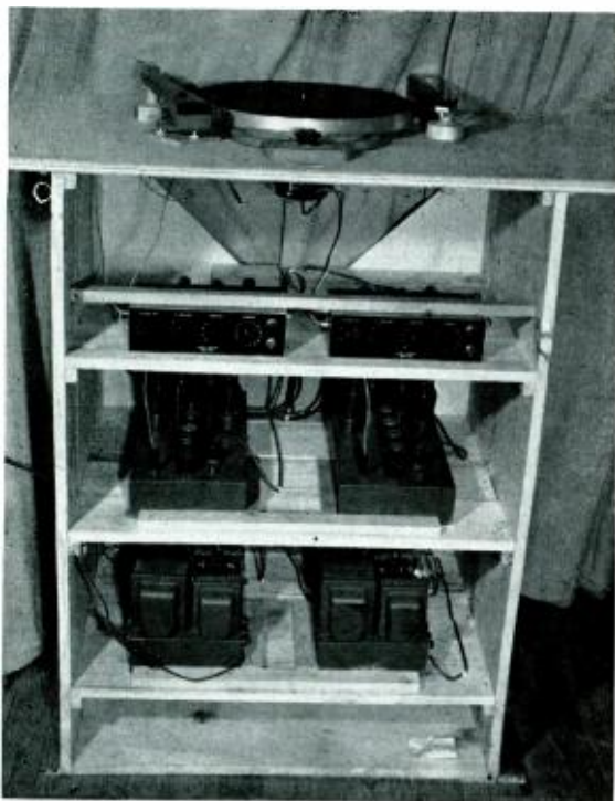
Fig. 5. Equipment includes two complete power amplifiers, two preamplifiers, two Gray pickup arms, and Rek-O-Kut turntable.
