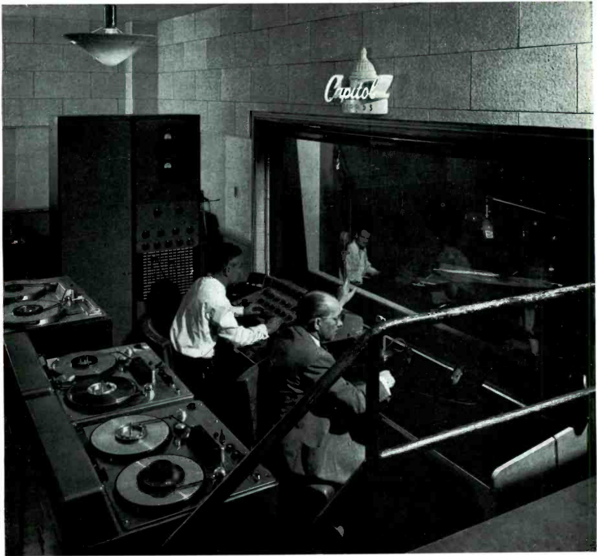
Control room setup for one of the Capitol recording studios. The Ampex tape machines, running at 15 inches per second, are operated remotely from the control position.
