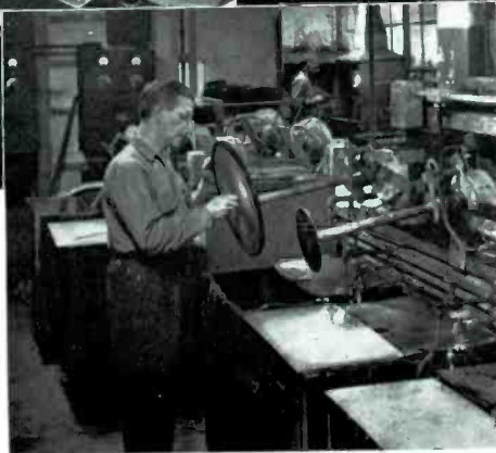
disc is being plated in preparation for pressing further test masters from it—an operation shown in the photo at the upper right.
