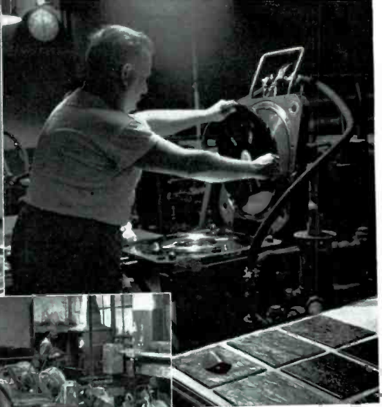
disc is being plated in preparation for pressing further test masters from it—an operation shown in the photo at the upper right.
