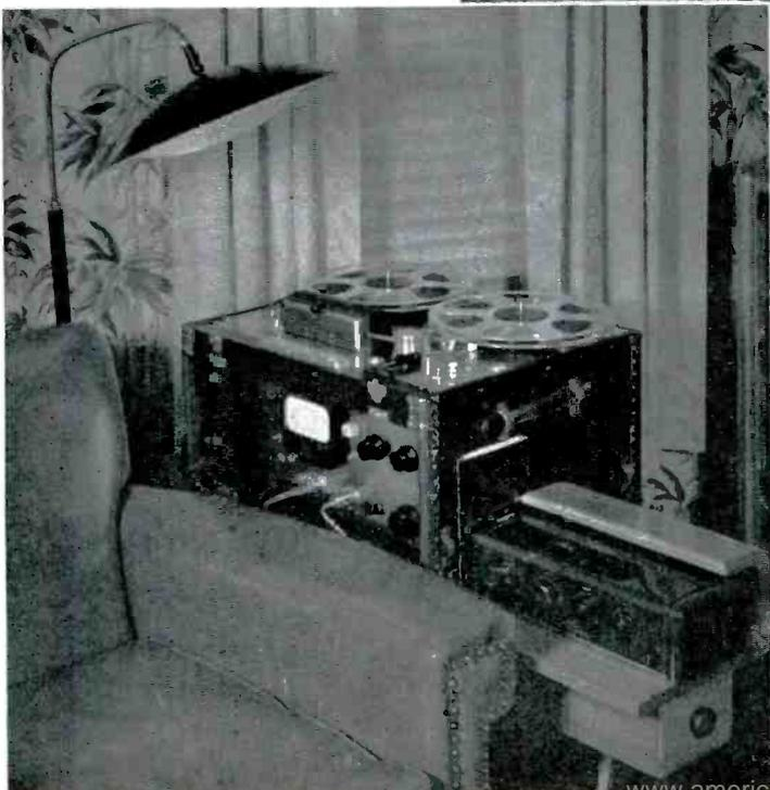
provided housing for the Altec 604-B with about 30 cu. ft. of closed baffle space and, directly below, enough space for the Radio Craftsmen TV tuner. The remaining equipment consists of a Garrard changer, RC-10 tuner, Ampex 400 recorder, Brook 10-watt amplifier, and a Shure 55-S microphone. Needless to say, the expanse of leather armchair next to the Ampex houses yours truly at practically every leisure moment."
