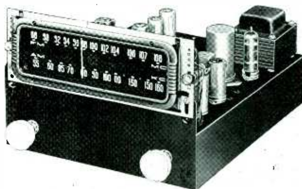
Bogen model R604 FM-AM tuner. Controls: tuning and selector. Latter provides AM, FM, power off, and two spares. Automatic frequency control incorporated; may be disabled by external switch. Armstrong circuit.
