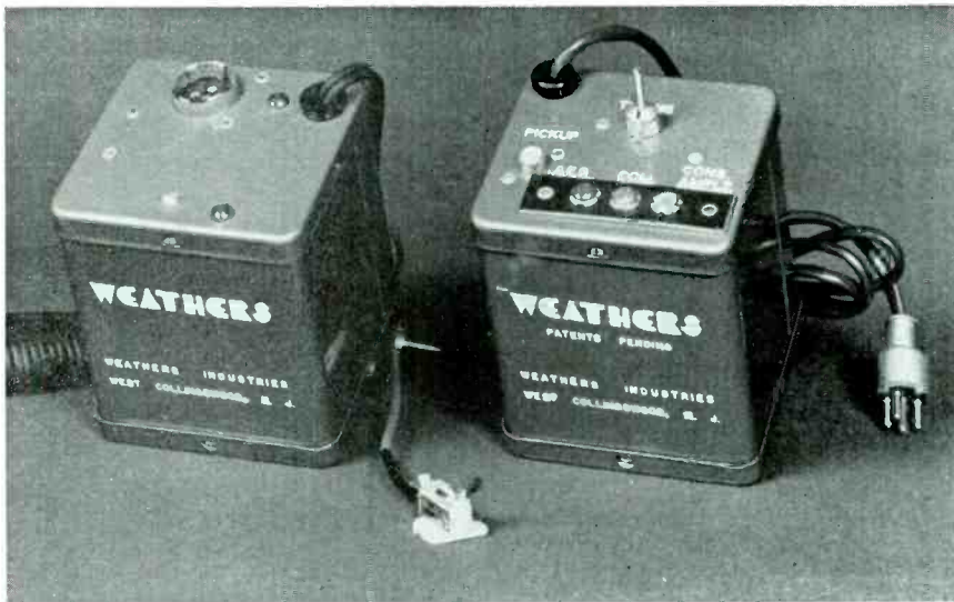
Fig. 2. The oscillator is shown at the right; accessory power supply at the left.
