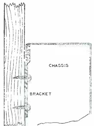
Fig. 5, above. Tuner and preamplifier chassis are hooked over brackets.
