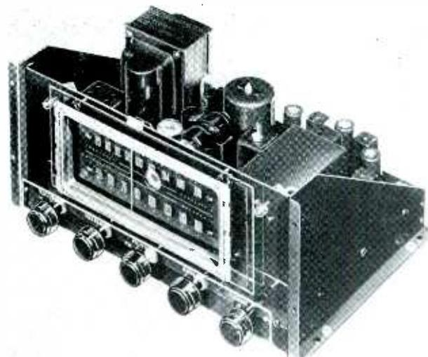
Sargent-Raymont model SR-51 FM-AM tuner. Controls: volume; bass and treble tone controls; tuning; input selector which provides two spares. Ratio detector.
