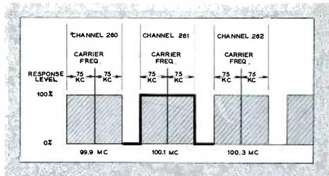
Fig. 2. The frequency response characteristics of the ideal tuner would exactly match those of the broadcast station, shown in Fig. 1 and indicated above by the heavy line.
