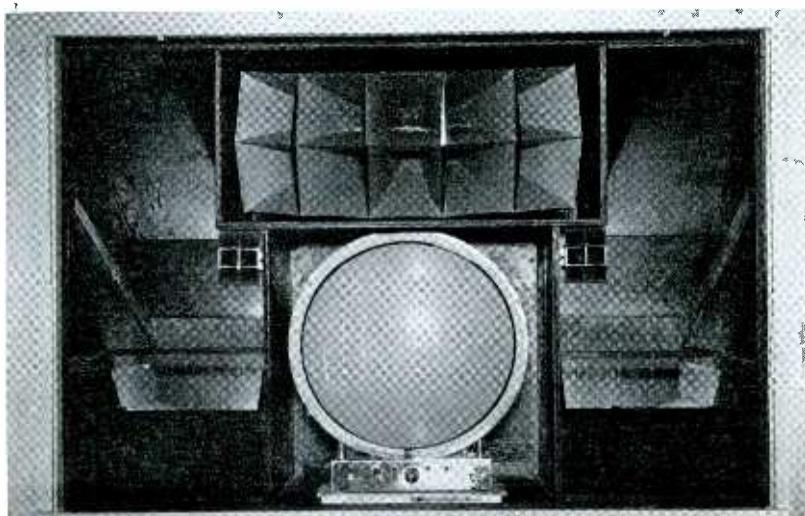
*This loudspeaker system was described in detail in HIGH-FIDELITY No. 4. It is shown again in this article because it represents close to if not the ultimate in sound reproduction, and because it utilizes the Klipsch principles normally applied to corner horns of the type illustrated on the preceding pages.*
