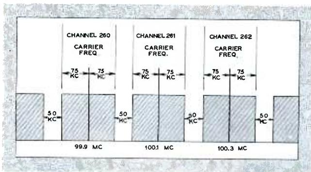
Fig. 1. Channels used by FM broadcast stations are centered around a carrier frequency with a 75 kilocycle band on either side of the carrier. A 50-kc. band separates channels.
