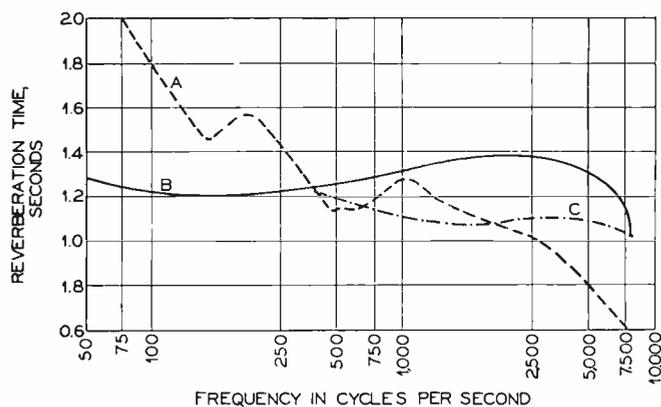
Fig. 3. Effect of acoustic treatment on reverberation time. Curve A: before treatment. B: after treatment, no carpet. C: carpet added.
