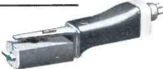
Plug-in magnetic head for Garrard record changer. Uses Audax polyphase principal. A simple twist brings either the standard or microgroove stylus into play. Sapphire stylii. Fine reproduction. Only 6-8 grams stylus point pressure. **1715**
