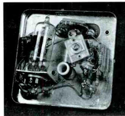
Fig. 3. View of underside of oscillator chassis. Tube at left is 6AT6. Almost in center is oscillator coil, which is slug tuned. Trimmer capacitor is just above coil.
