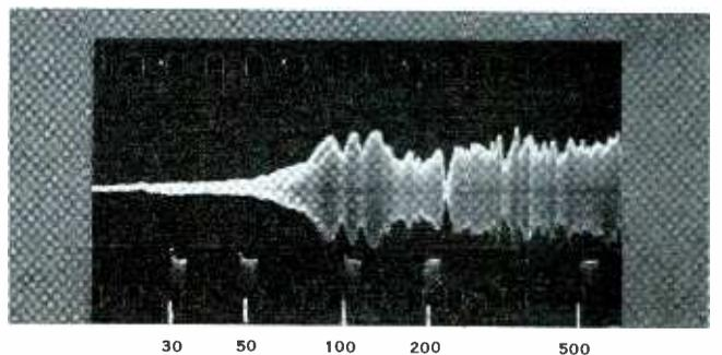
Fig. 12. Same as Fig. 11, but cabinet placed 4 ft. from corner. The more central position shows room reflections at about 100 cycles. The 40-cycle hump of Fig. 11 has disappeared.
