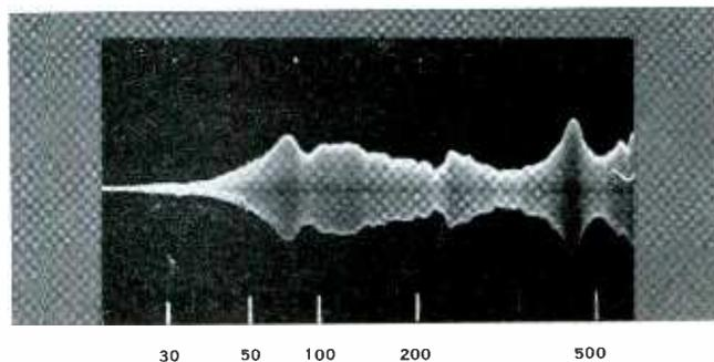
Fig. 14. Speaker mounted as for Fig. 11 but taken outside for free field response. There is obviously a complete absence of room effects. The main cone-cabinet resonance occurs at 75 cycles. Some frequency doubling, but less than shown in Fig. 10.
