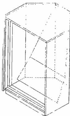
*At the left is pictured a typical, medium size corner enclosure. It is intended for use either with a single speaker, preferably of the coaxial type, or with two speakers, one of which is a tweeter. The sketch gives an idea of internal construction.*
