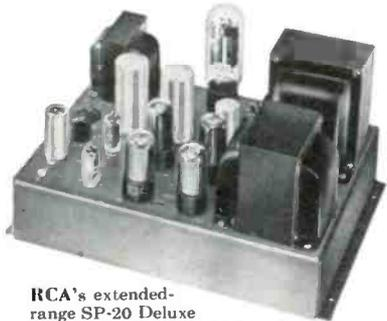
RCA's extended-range SP-20 Deluxe 20-watt amplifier for fidelity at its highest. Straight-line response 20-20,000 cycles
