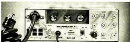
McIntosh C-8, showing new input and rear-panel control setup.
