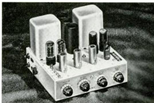
The A 20C amplifier gives 20 clean watts from low-cost tubes.
