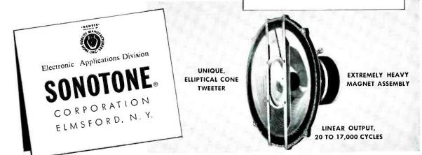
SONOTONE CA-15 COAXIAL SPEAKER has a huge 5-lb. Alnico V magnet, with 15.000 gauss flux density. Unusual velour suspension of the ridged, curvilinear cone drops resonance to 30 cycles, keeps extreme "lows" full, rich and natural. The six-inch non-metallic cone tweeter is elliptical, providing wide lateral dispersion of "bighs" without tinniness or piercing effect. 25 watt output, 40 watt peak. Woofer and tweeter also available individually.
