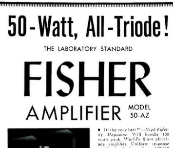
ode amplifier. Uniform response within 1 db from 5 to 100,000 cycles. Less than 1% distortion at 50 watts, Ilum and noise content 96 db below full output-virtually non-measurable! Oversize components and quality workmanship in detail. Includes FISHER everv Z-MATIC, at no additional cost. \$159.50
