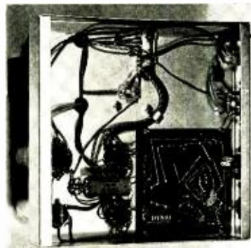
Bottom view shows completed wiring.
