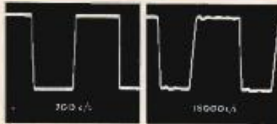
Square wave response at 300 c.p.s. fundamental and 15,000 c.p.s. fundamental; the latter contains harmonics to about 150,000 cycles and indicates the degree of damping attained.
