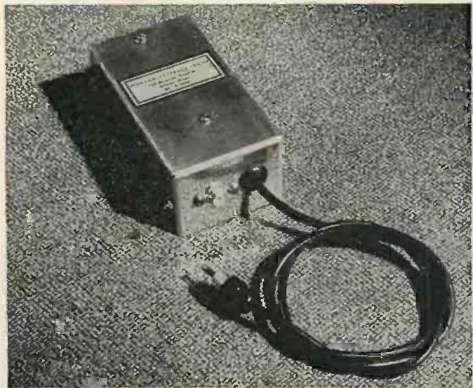
The booster connects between pickup and preamp.
