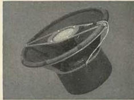
12" RF-471 . . . \$49.95 • Coaxial mounting of tweeter and woofer. Frequency response 30 to 14,000 cps. Power-handling capacity, 32 watts program material. Better than 100 degrees angle of coverage. Aluminum spider and Carpinchio leather suspension. 20 ounce Alnico V low-frequency and 2.15 ounce Alnico V high-frequency unit magnets.
