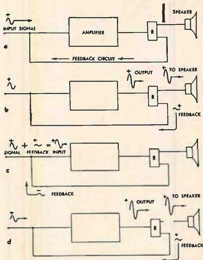
Fig. 1. In a positive feedback circuit, the portion of output signal that is fed back to the input adds to the input signal, increasing the amplifier's gain as well as its distortion.
