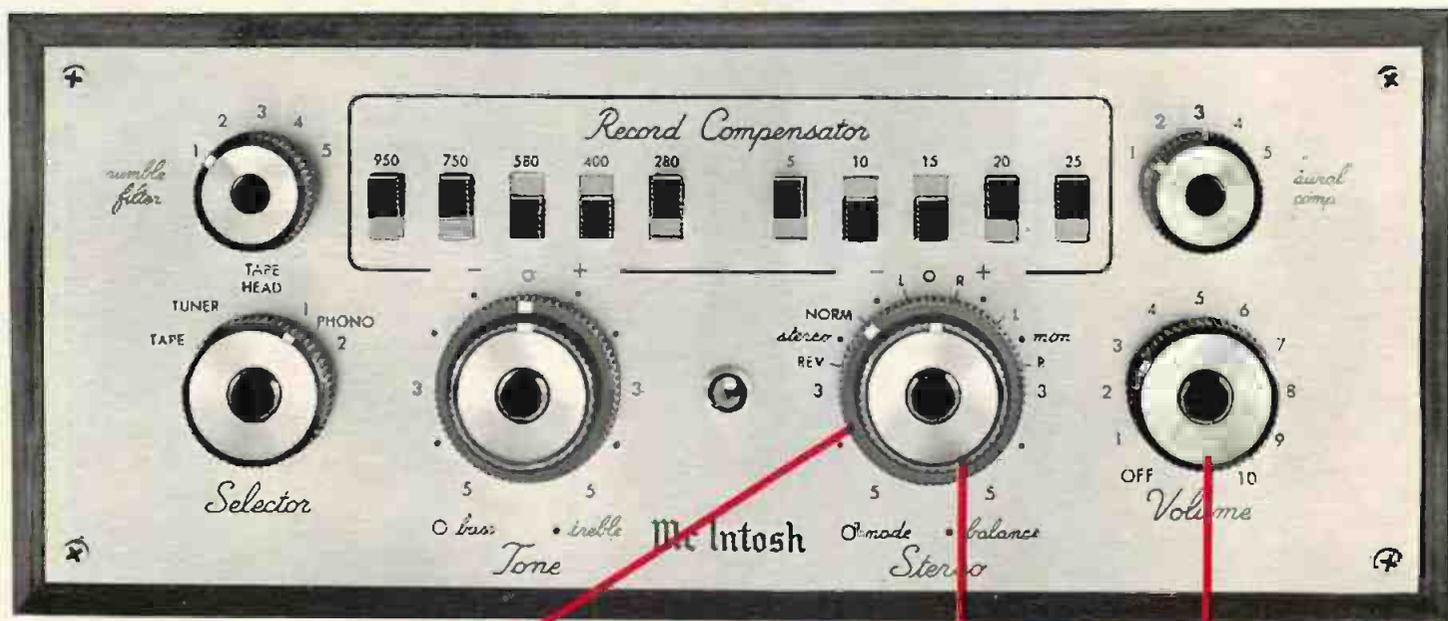
STEREO MODE SELECTOR      STEREO BALANCE      STEREO MASTER VOLUME
