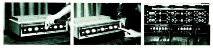
The Continuously Variable Loudness Control is on exclusive feature of the Carillon Stereo Amplifier. It automatically compensates for base and treble at low listening levels; Single Knob Balance outomotically adjusts the volume level between speakers.
