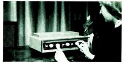
Here's how Bell makes it easy for you to enjoy your new Carillon Stereo Amplifier: Built-in Pre-Amplifiers mean that all operating controls can be located on the front panel of the amplifier, so they became part of one compact unit. Separate Base and Treble Tane Controls are provided for both right and left channels. As shown here, each can be individually adjusted for greatest listening enjoyment.
