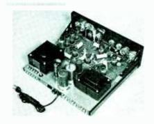
Upper view of completed unit. The tubes have been installed, but not the cover.
