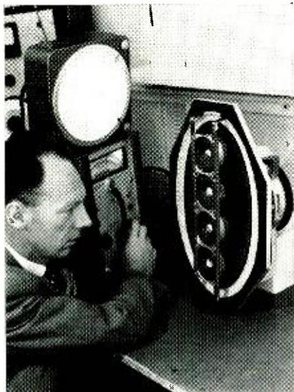
*Strobe tests cone movement at EMI.*
