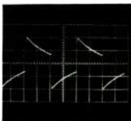
Square-wave response to 50 cps, left, and to 10 kc at average and higher settings of volume control.
