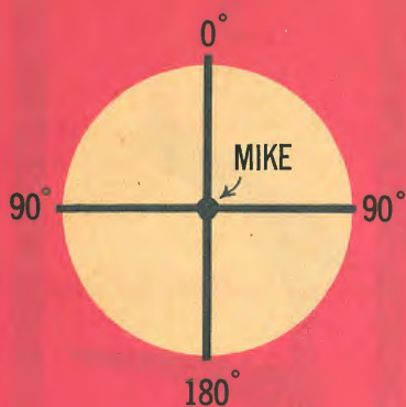
OMNIDIRECTIONAL One side of diaphragm is exposed to air.
