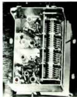
SUPER-SYNCHRODE** FRONT END WITH THREE FIELD EFFECT* TRANSISTORS PROVIDES A TUNER SENSITIVITY OF 1.8 MICROVOLTS (IHF).
